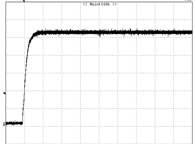
Figure 16 – Start-up Profile, 230 VAC 2 V, 20 ms / div.
