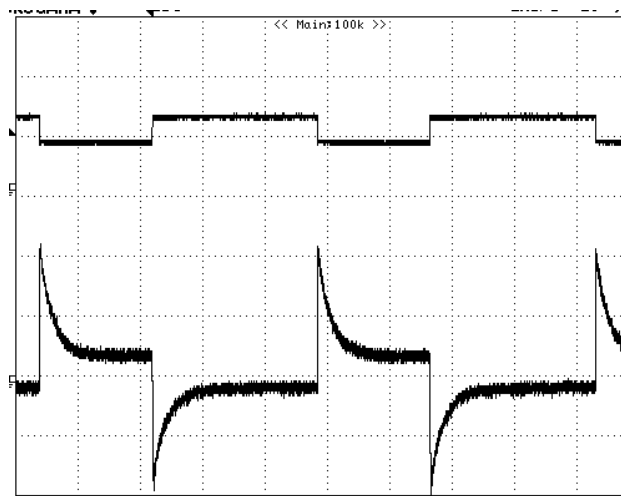
Figure 20 – Transient Response, 230 VAC, 50-100-50% Load Step. Upper: Load Current, 0.5 A / div. Bottom: Output Voltage 200 mV, 10 ms / div.
