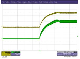
Figure 17 – Start-up Profile, 90 VAC. Upper:  $V_{5 V}$ , 2 V / div. Lower:  $V_{14.5 V}$ , 5 V, 5 ms / div.
