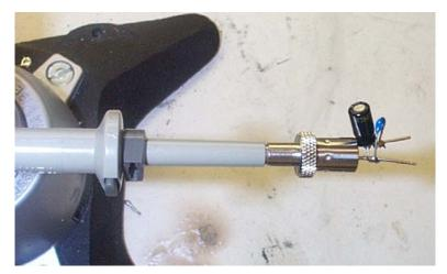
Figure 27 – Oscilloscope Probe with Probe Master (<u>www.probemaster.com</u>) 4987A BNC Adapter (modified with wires for ripple measurement and two parallel decoupling capacitors added).
