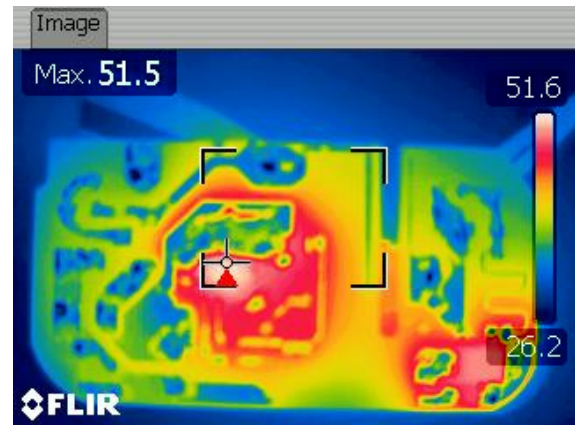
Figure 10 – Thermal Image of Assembly (Bottom) V_{IN} : 265 VAC, Full Load, LinkSwitch-II is Highest Recorded Temperature at 51.5 °C.
