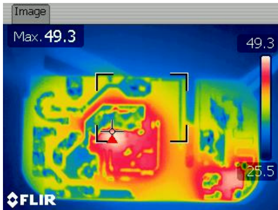
Figure 9 – Thermal Image of Assembly (Bottom) V_{IN} : 85 VAC, Full Load, LinkSwitch-II is Highest Recorded Temperature at 49.3 °C.
