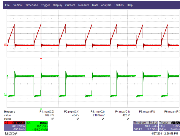
Figure 48 – 185 VAC, 50 Hz. Upper: I DRAIN , 0.2 A / div. Lower: V DRAIN , 100 V / div., 5 μs / div.
