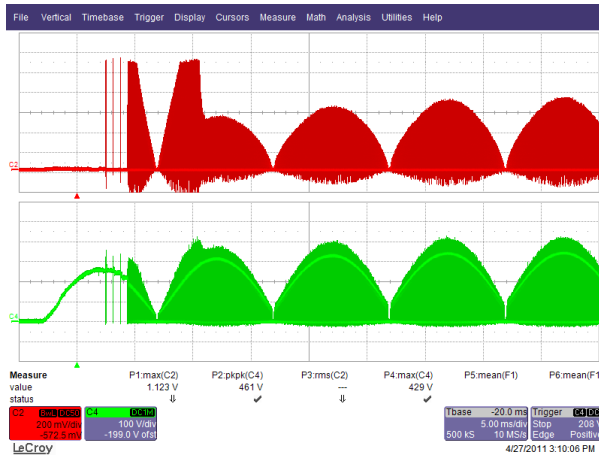
Figure 51 – 185 VAC, 50 Hz, 0° Phase Start-Up. Upper: I_{DRAIN} , 200 mA / div. Lower: V_{DRAIN} , 100 V, 5 ms / div.
