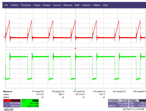
Figure 50 – 265 VAC, 50 Hz. Upper: I DRAIN , 0.2 A / div. Lower: V DRAIN , 100 V / div., 10 μs / div.
