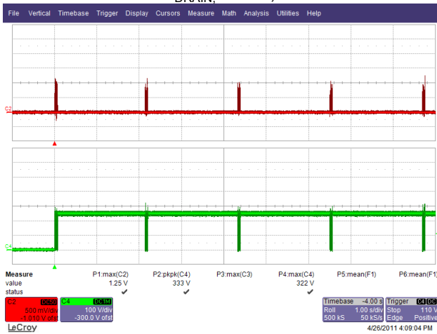
Figure 61 – 185 VAC, 50 Hz Output Short Condition. Upper: I_{DRAIN} , 500 mA / div. Lower: V_{DRAIN} , 100 V, 1 s / div.
