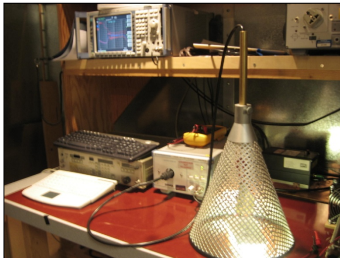
Figure 69 – Conducted EMI Test Set-Up.
