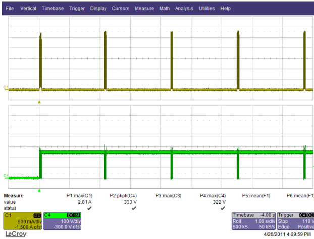
Figure 59 – 185 VAC, 50 Hz Output Short Condition. Upper: I_{OUT} , 500 mA / div. Lower: V_{DRAIN} , 100 V, 1 s / div.
