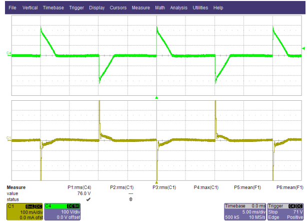
Figure 38 – 230 VAC, 45° Conduction Angle. Upper: V_{IN} , 100 V / div. Lower: I_{IN} , 100 mA, 10 ms / div.
