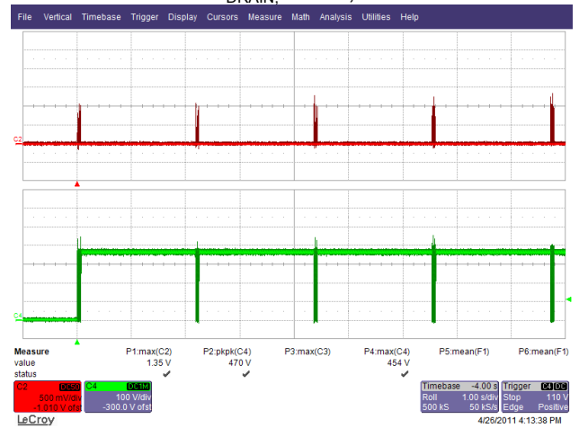
Figure 62 – 265 VAC, 50 Hz Output Short Condition. Upper: I_{DRAIN} , 500 mA / div. Lower: V_{DRAIN} , 100 V, 1 s / div.
