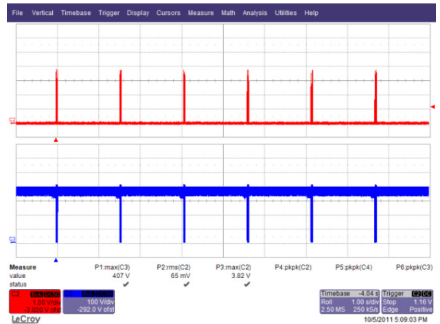
Figure 62 – 265 VAC, 50 Hz Output Short. Upper: I_{DRAIN} , 1 A / div. Lower: V_{DRAIN} , 100 V, 1 s / div.
