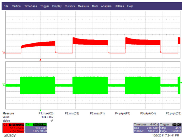
Figure 8 – 90 VAC, 0 - 90 VAC Line Transient. Upper: I_{OUT} , 50 mA / div. Lower: V_{IN} , 100 V, 2 s / div.
