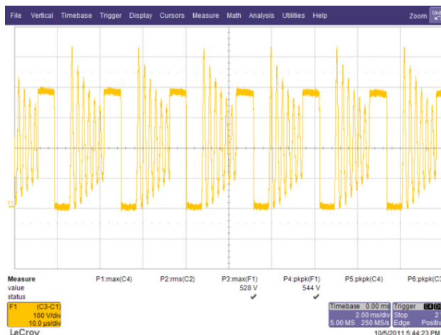
Figure 66 – 265 VAC, 50 Hz Normal Operation. PIV: 200 V, 10 \mu s / div.
