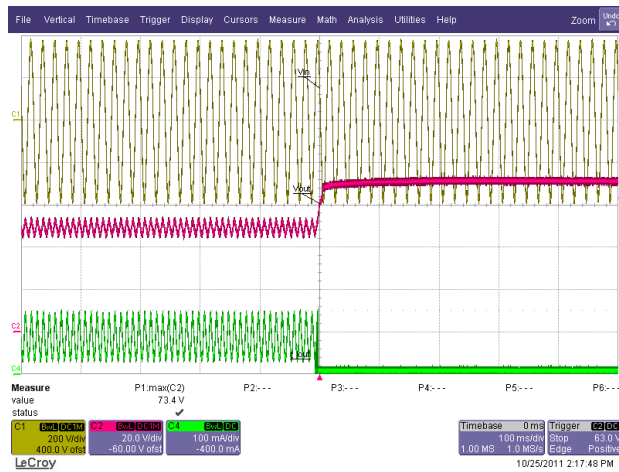
Figure 38 – 265 VAC / 50 Hz, Normal Operation then No-load. Ch1: V_{IN} , 200 V / div. Ch2: V_{OUT} , 20 V / div. Ch4: I_{OUT} , 100 mA / div., 100 ms / div.
