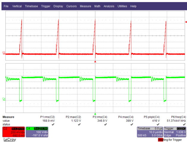
Figure 48 – 265 VAC, 50 Hz. Upper: I_{DRAIN} , 0.1 A / div. Lower: V_{DRAIN} , 100 V / div., 10 \mu s / div.
