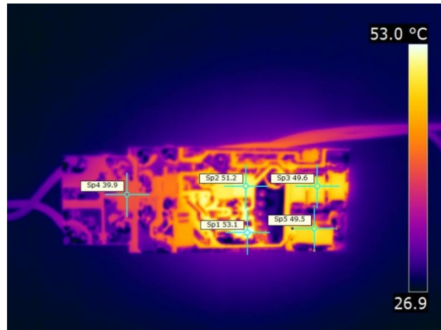
Figure 26 – Bottom Side. R4- Current Sense Resistor: 53.1 °C.
