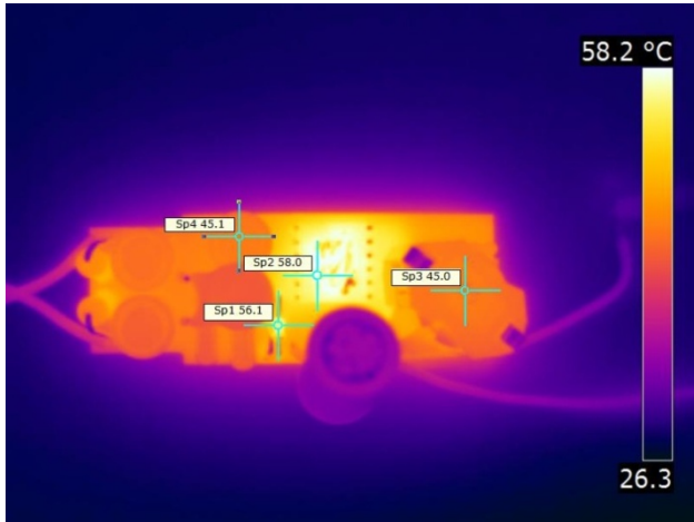
Figure 23 – Top Side. U1- LNK460VG: 58 °C.
