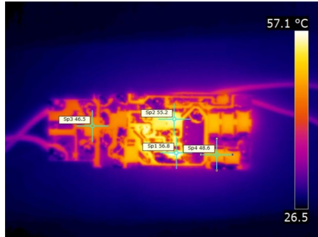
Figure 24 – Bottom Side. R4- Current Sense Resistor: 56.8 °C.
