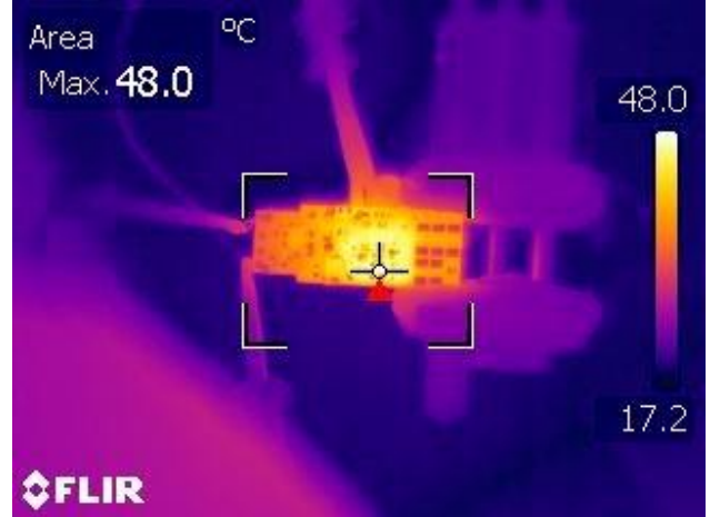
Figure 17 – Bottom Side. R4- Current Sense Resistor: 48 °C.
