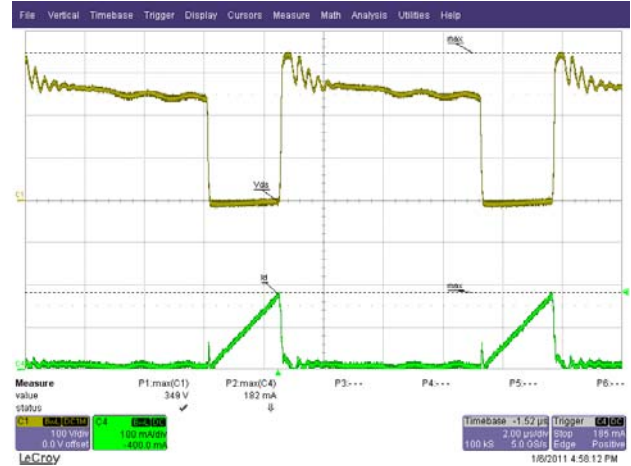
Figure 28 – 115 VAC / 60 Hz, LED = 3 V / 366 mA. Upper: V_{DRAIN} , 100 V / div., 2 \mu s / div. Lower: I_{DRAIN} , 0.1 A / div.
