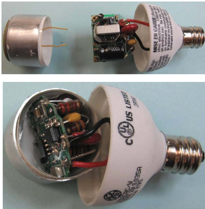
Figure 3 – RD-268 Driver Board Removed and Inserted into a Typical Candelabra Base (Metal Part Forms LED Heat Sink).
