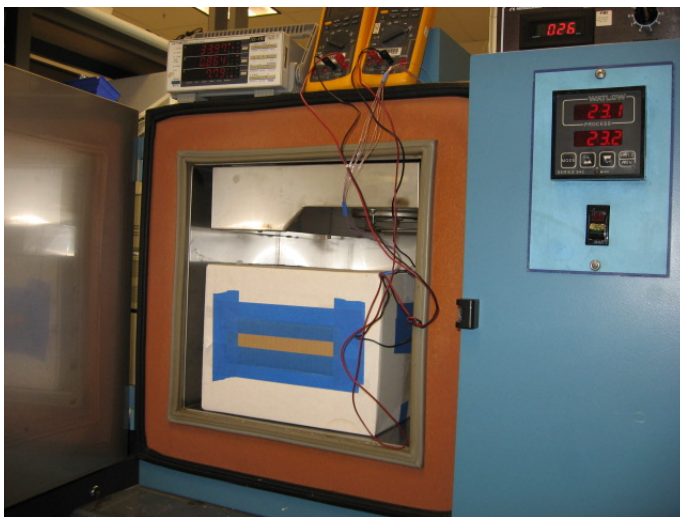
Figure 19 – Thermal Chamber Set-up Showing Box Used to Prevent Airflow Over UUT.
