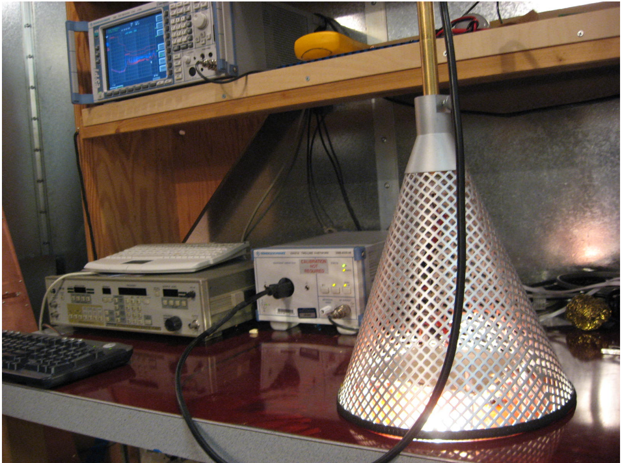
Figure 67 – EMI Test Set-up.
