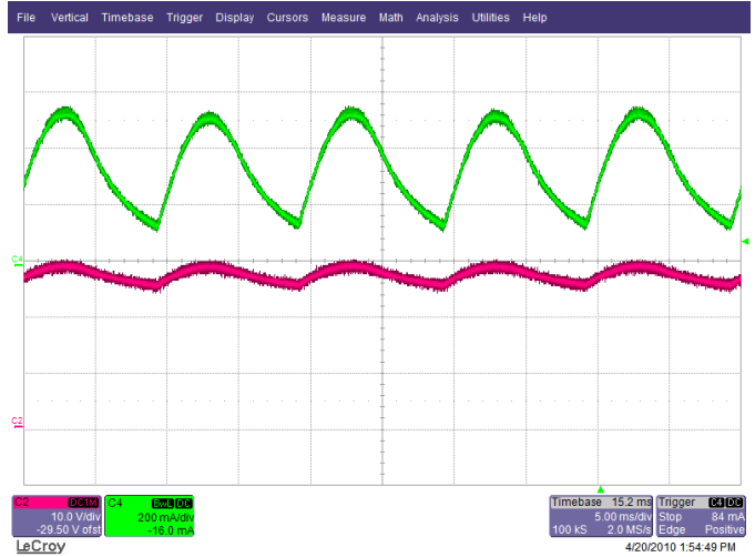
Figure 22 – 265 VAC, Full Load. Upper: I_{RIPPLE} , 0.2 A / div. Lower: V_{OUT} , 10 V, 5 ms / div.
