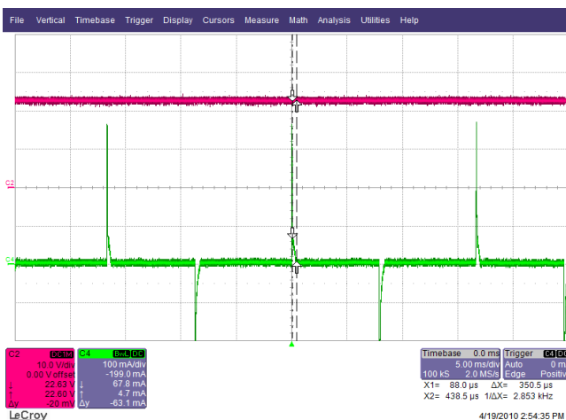
Figure 33 – 115 VAC, 8° Phase. Upper: V_{OUT} , 10 V / div. Lower: I_{IN} , 0.1 A / div., 5 ms / div.
