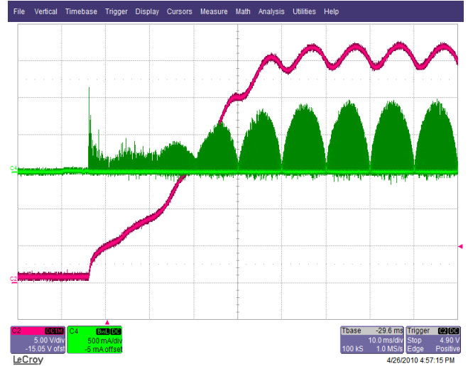
Figure 24 – 265 VAC, Full Load. Upper: I_{RIPPLE} , 0.5 A / div. Lower: V_{OUT} , 5 V, 10 ms / div.
