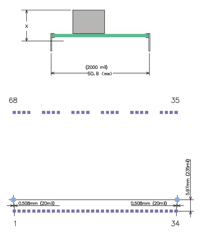
Fig. 3 Side view (top) / Mechanical fixing (bottom) 6SD106EI
