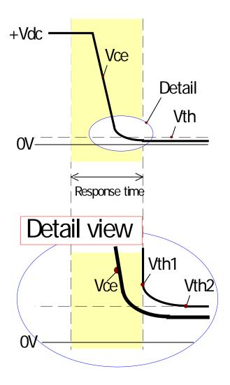
Fig. 5 Collector-sense voltage curve
