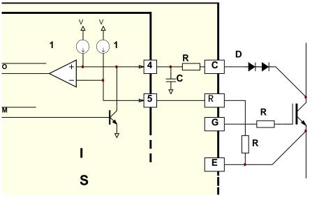
Fig. 4 Collector-sense circuit principle
