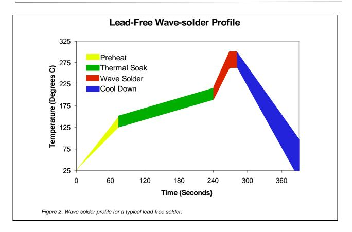
lead-free solder profile is noticeably longer than the equivalent stage for the leaded solder. The longer soak time is required to ensure that the components to be soldered have reached their higher pre-solder temperature.
