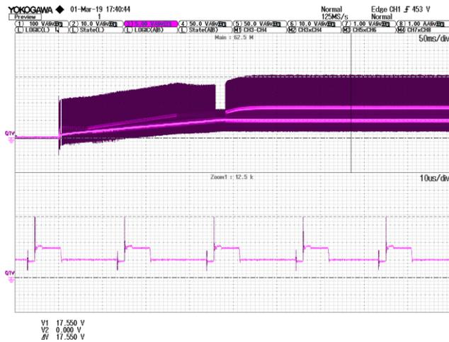
**Figure 45** – Q1 Selection MOSFET Voltage Waveforms, 265 VAC Input.
