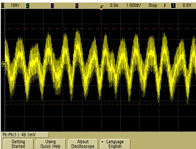
**Figure 70** –  $V_{IN} = 230 \text{ VAC}$ .  $V_{RIPPLE\_CV1} = 49.1 \text{ mV}_{PK-PK}$ .
