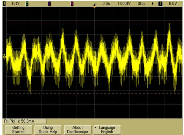
**Figure 66** –  $V_{IN} = 115 \text{ VAC}$ .  $V_{RIPPLE\_CV1} = 50.3 \text{ mV}_{PK-PK}$ .
