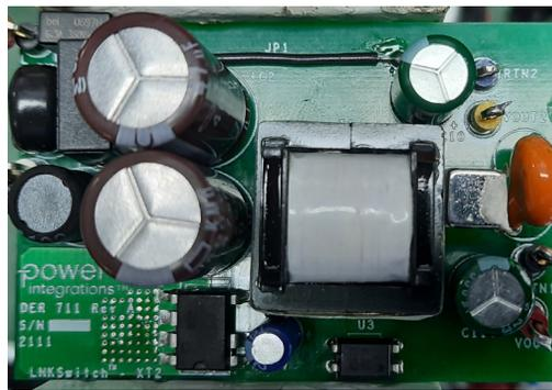
**Fig. 3 DER-711 (TOP VIEW) with permanent magnet placed on transformer core.**
