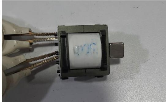
**Fig.1 A permanent magnet is placed next to the transformer while the primary inductance is being measured (magnet orientation #1).**
