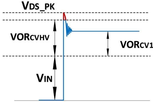
Fig. 2 Peak drain-source voltage on the primary switch when SEL FET is on
