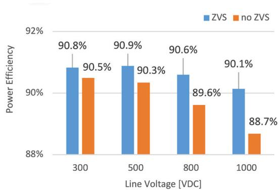
Fig. 11 Efficiency improvement with ZVS
