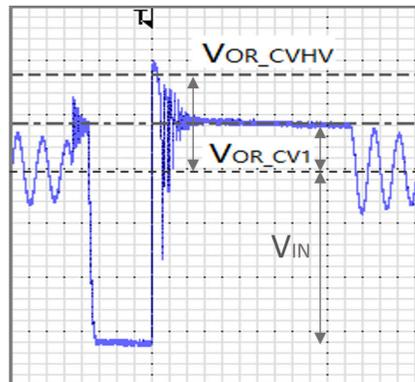
Fig. 7 Primary switch transient drain-source voltage,  $V_{DS\text{PK}} > V_{OR\text{CVHV}} + V_{IN}$ , with overspill effect
