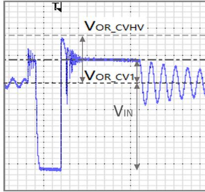
Fig. 8 Primary switch transient drain-source voltage,  $V_{DS\text{PK}} < V_{OR\text{CVHV}} + V_{IN}$ , no overspill effect
