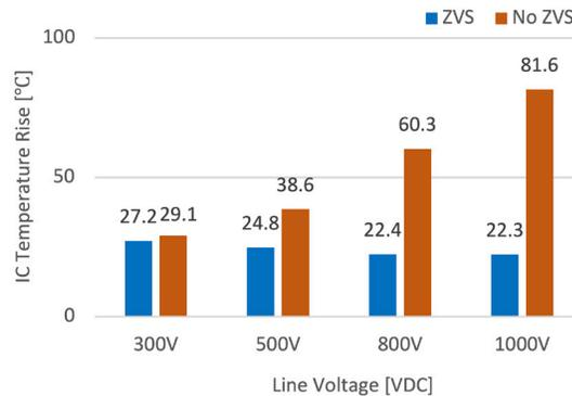
Fig. 12 IC temperature rise improvement with ZVS, tested at room temperature 25 °C
