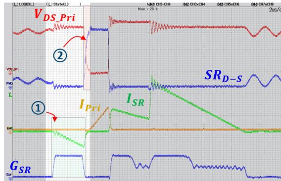
Fig. 4 ZVS waveform
