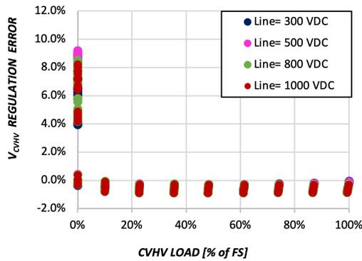
Fig. 9 CVHV output voltage regulation with overspill effect, 0 percent -100 percent load on CV1 (5 V) & CV2 (24 V)
