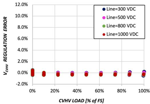
Fig. 10 CVHV output voltage regulation with no overspill effect, 0 percent - 100 percent load on CV1 (5 V) & CV2 (24 V)
