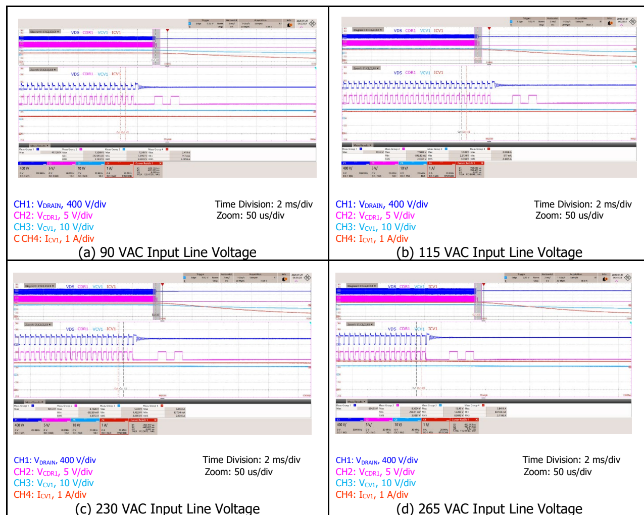
Figure 36 - CV1 Overload Protection at 90, 115, 230 and 265 VAC.
