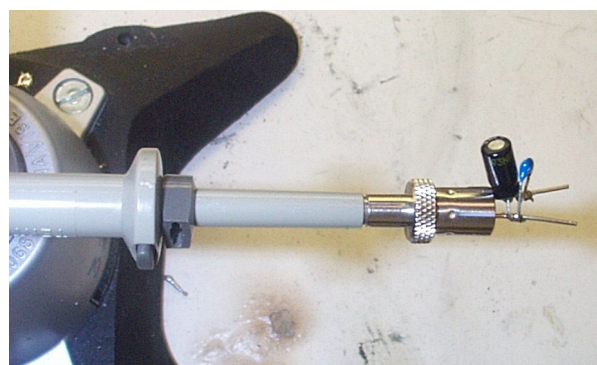
Oscilloscope Probe with Probe Master (www.probemaster.com) 4987A BNC Adapter. (Modified with wires for ripple measurement, and two parallel decoupling capacitors added)
