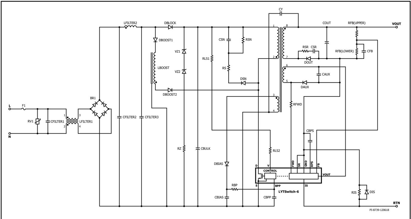
Figure 2. Typical Application Schematic for  $V_o > 24 V$ .
