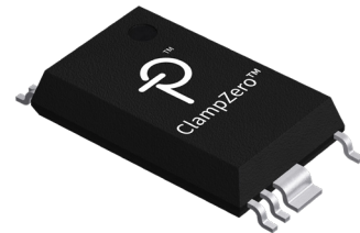
Figure 2. MinSOP-16A Package with Creepage for High-Side Driver.
