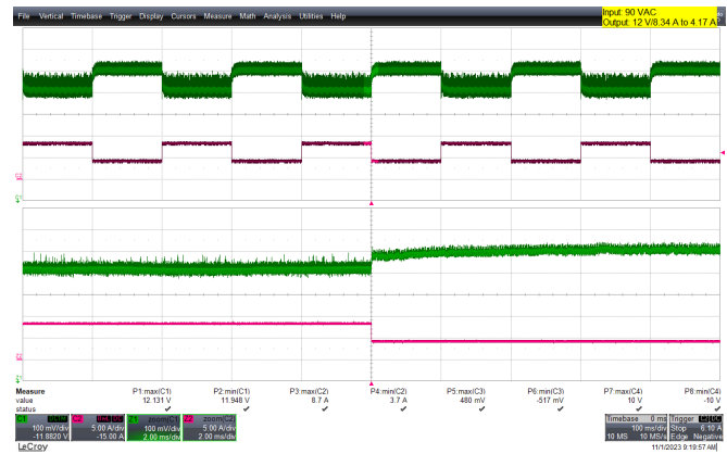
Figure 54 – 90 VAC 60 Hz. I_{OUT} = 8.34\text{ A} - 4.17\text{ A} (100 - 50%) Load Step.
