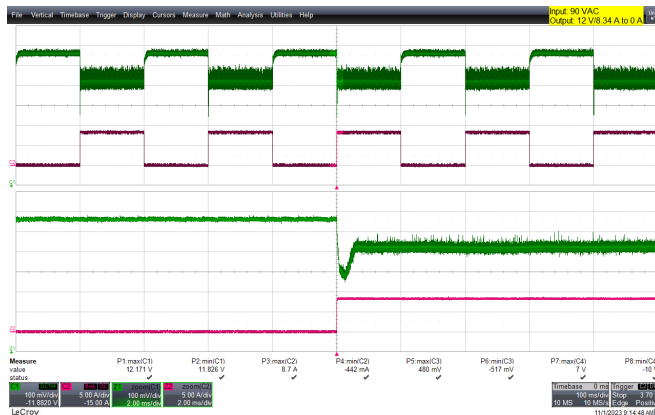
Figure 49 – 90 VAC 60 Hz. I_{OUT} = 0\text{ A} - 8.34\text{ A} (0 - 100%) Load Step.
