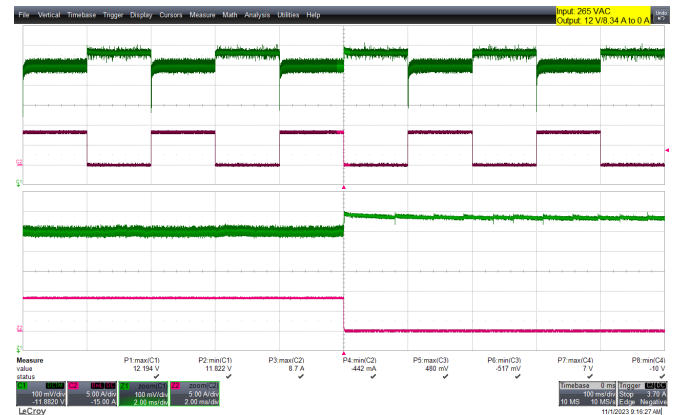
Figure 52 – 265 VAC 50 Hz. I_{OUT} = 8.34\text{ A} - 0\text{ A} (100 - 0%) Load Step.
