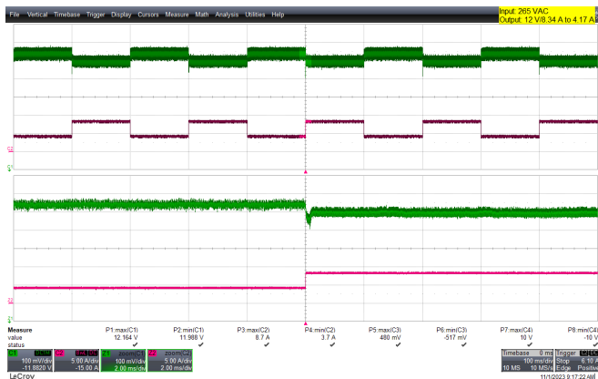
Figure 55 – 265 VAC 50 Hz. I_{OUT} = 4.17\text{ A} - 8.34\text{ A} (50 - 100%) Load Step.
