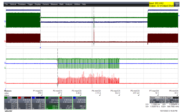
Figure 66 – 265 VAC, I_{OUT} = Output Shorted.
