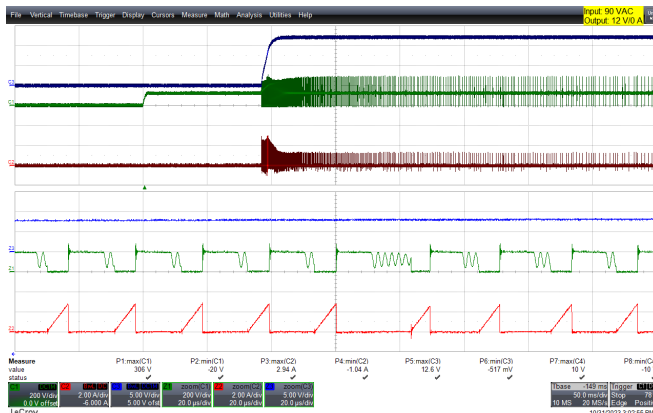
Figure 59 – 90 VAC, I_{OUT} = 0 A (No-Load).
