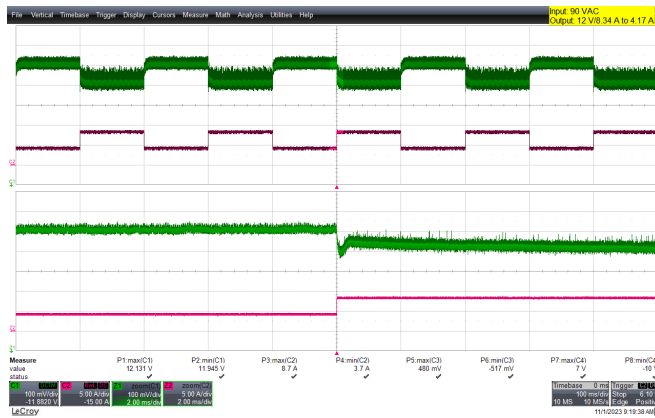
Figure 53 – 90 VAC 60 Hz. I_{OUT} = 4.17\text{ A} - 8.34\text{ A} (50 - 100%) Load Step.
