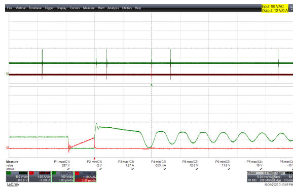
Figure 63 – 90 VAC, I_{OUT} = 0 A (No-Load). CH1: Drain Voltage: 100 V / div, 5 ms / div. CH2: Drain Current: 1 A / div, 5 ms / div. Zoom: 3 \mu s / div. Drain voltage, Max. = 287 V. Drain current, Max. = 1.27 A.
