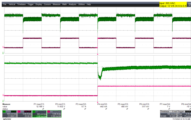
Figure 51 – 265 VAC 50 Hz. I_{OUT} = 0\text{ A} - 8.34\text{ A} (0 - 100%) Load Step.
