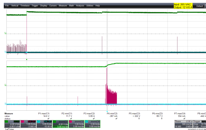
Figure 113 – 265 VAC, I_{OUT} = 0 A (No-Load). OVP Running Short CH 1: Output Voltage: 4 V / div, 500 ms / div. CH 2: Drain Current: 1 A / div, 500 ms / div. CH 4: Output Current: 5 A / div, 500 ms / div. Max Output Voltage = 14.6 V
