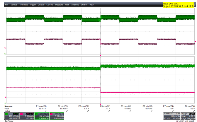
Figure 56 – 265 VAC 50 Hz. I_{OUT} = 8.34\text{ A} - 4.17\text{ A} (100 - 50%) Load Step.
