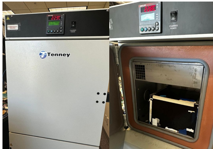
Figure 28 – Thermal Chamber Test Set-up.
