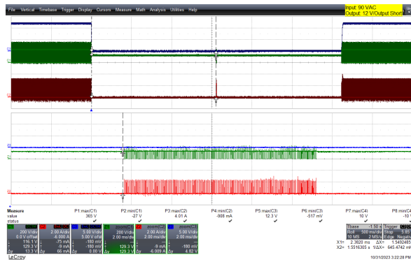
Figure 65 – 90 VAC, I_{OUT} = Output Shorted.
