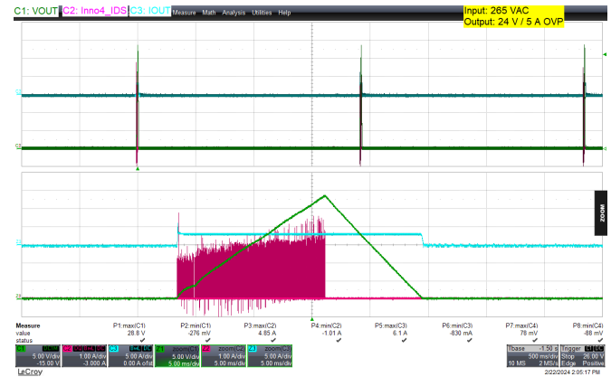
Figure 139 – 265 VAC, I_{OUT} = 5 A (Full-Load). OVP Startup CH 1: Output Voltage: 4 V / div, 500 ms / div. CH 2: Drain Current: 1 A / div, 500 ms / div. CH 4: Output Current: 5 A / div, 500 ms / div. Max Output Voltage = 28.8 V
