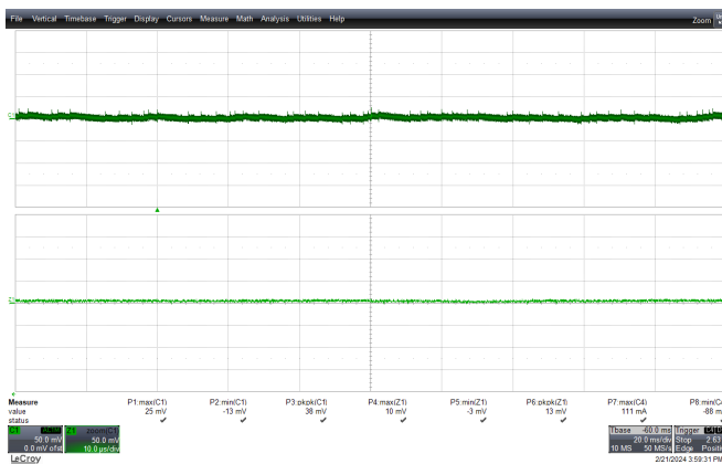
Figure 131 – Output Ripple. (PK-PK – 38 mV). 230 VAC Input, 0% Load. V_{OUT\_RIPPLE} , 50 mV / div, 20 ms / div. Zoom: 10 \mu s.
