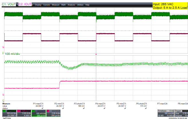
Figure 59 – 265 VAC 50 Hz. I_{OUT} = 2.5\text{ A} - 8.34\text{ A} (50 – 100%) Load Step.
