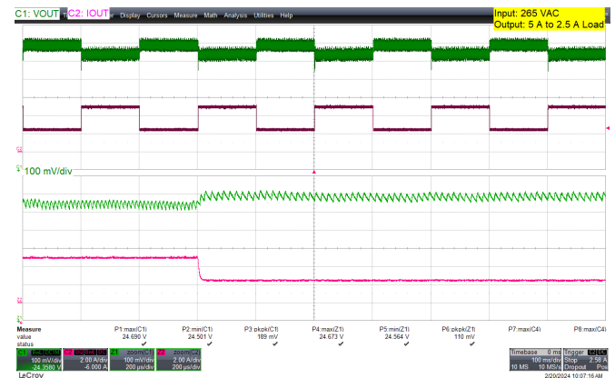
Figure 60 – 265 VAC 50 Hz. I_{OUT} = 8.34\text{ A} - 2.5\text{ A} (100 – 50%) Load Step.
