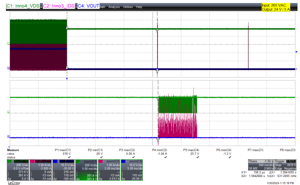
Figure 78 – 265 VAC, I_{OUT} = Output Shorted.
