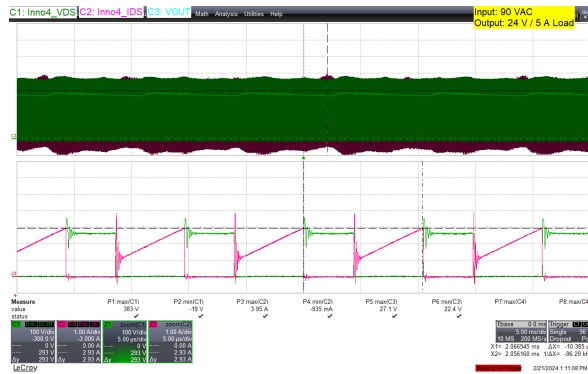
Figure 73 – 90 VAC, I_{OUT} = 5 A (Full-Load).
