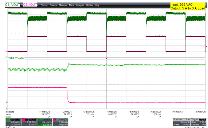
Figure 56 – 265 VAC 50 Hz, I_{OUT} = 5\text{ A} - 0\text{ A} (100 – 0%) Load Step.
