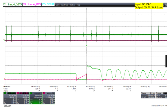
Figure 75 – 90 VAC, I_{OUT} = 0 A (No-Load).
