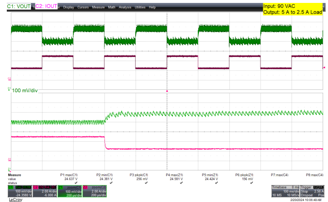
Figure 58 – 90 VAC 60 Hz. I_{OUT} = 5\text{ A} - 2.5\text{ A} (100 – 50%) Load Step.
