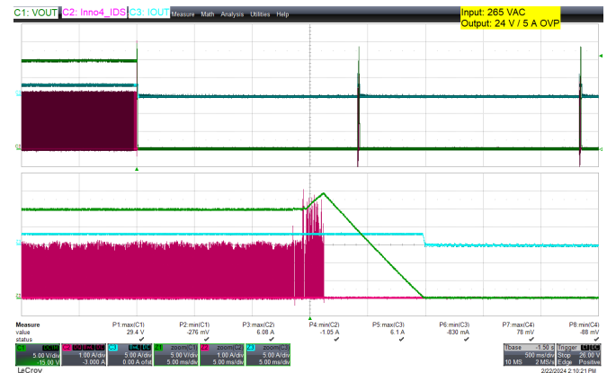
Figure 135 – 265 VAC, I_{OUT} = 5 A (Full-Load). OVP Running Short CH 1: Output Voltage: 5 V / div, 500 ms / div. CH 2: Drain Current: 1 A / div, 500 ms / div. CH 4: Output Current: 5 A / div, 500 ms / div. Max Output Voltage = 29.4 V
