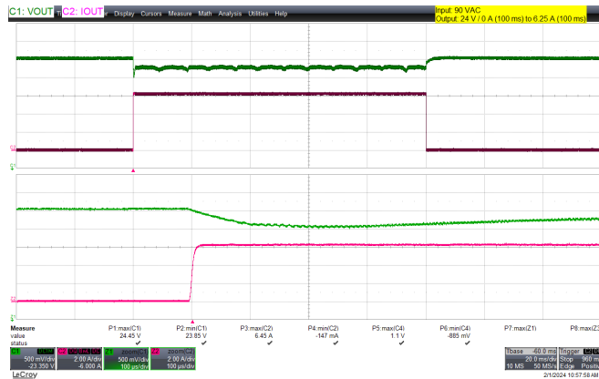
Figure 65 – 90 VAC 60 Hz. I_{OUT} = 0 A (100ms) – 6.25 A (100 ms) - (0 – 125%) Load Step. CH1: Output Voltage: 500 mV / div, 20 ms / div. CH2: Output Current: 2 A / div, 20 ms / div. Zoom: 100 \mu s / div. V_{OUT\_MAX} : 24.5 V. V_{OUT\_MIN} : 23.9 V.
