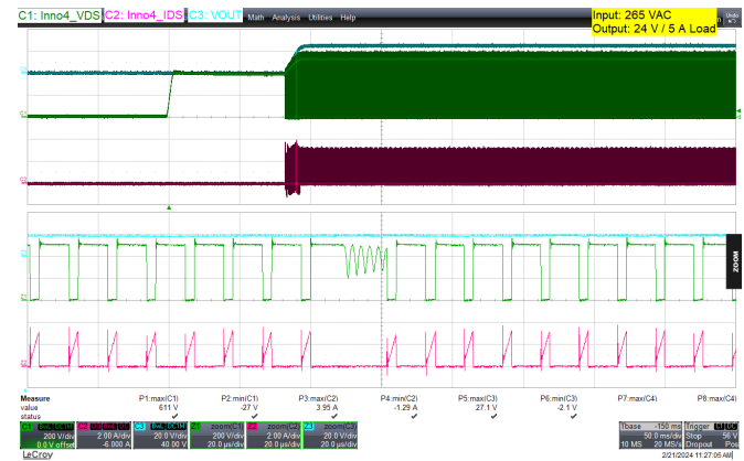
Figure 70 – 265 VAC, I_{OUT} = 5 A (Full-Load). CH1: Drain Voltage: 200 V / div, 50 ms / div. CH2: Drain Current: 2 A / div, 50 ms / div. CH3: Drain Voltage: 20 V / div, 50 ms / div. Zoom: 20 \mu s / div. Drain voltage, Max. = 611 V. Drain current, Max. = 3.95 A.
