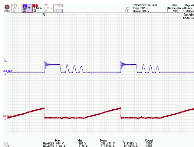
Figure 149 – InnoSwitch3-AQ Drain Voltage and Current. 80 VDC, 1.8 A Load, 25 °C Ambient.
