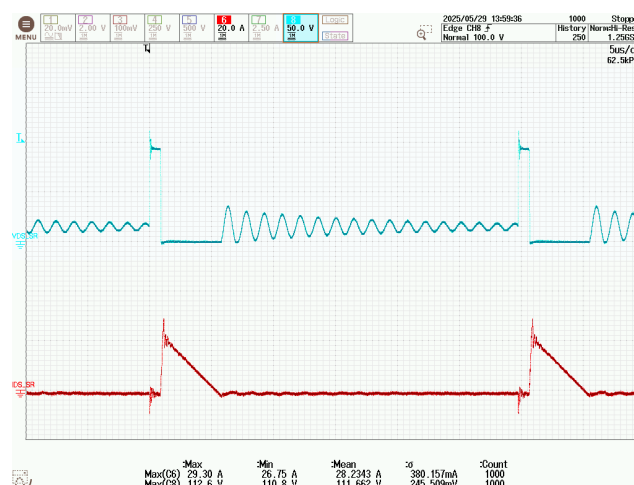
Figure 188 – SR FET Drain Voltage and Current. 1000 VDC, 1.8 A Load, -40 °C Ambient.
