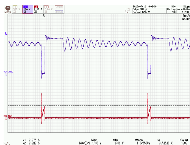
Figure 128 – InnoSwitch3-AQ Drain Voltage and Current. 1000 VDC, 1.8 A Load, 85 °C Ambient.
