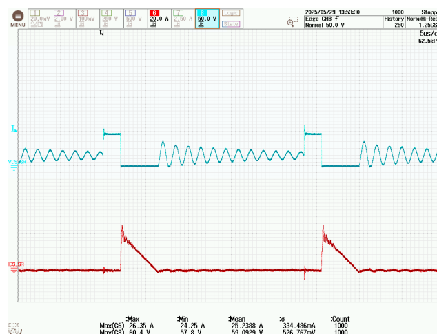
Figure 186 – SR FET Drain Voltage and Current. 400 VDC, 1.8 A Load, -40 °C Ambient.
