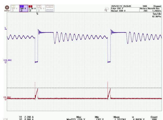
Figure 164 – InnoSwitch3-AQ Drain Voltage and Current. 1000 VDC, 2.33 A Load, 25 °C Ambient.
