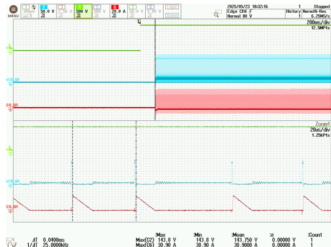
Figure 62 – SR FET Drain Voltage and Current. 1000 VDC, 6.43 \Omega Load. CH2: V_{DS(SR)} , 50 V / div. CH4: V_{IN} , 500 V / div. CH6: I_{D(SR)} , 20 A / div. Time: 200 ms / div.
