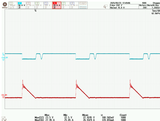
Figure 165 – SR FET Drain Voltage and Current. 80 VDC, 2.33 A Load, 25 °C Ambient. CH2: V_{DS(SR)} , 50 V / div. CH6: I_{D(SR)} , 20 A / div. Time: 5 \mu s / div.
