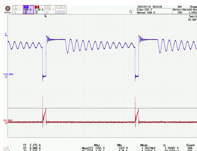
Figure 136 – InnoSwitch3-AQ Drain Voltage and Current. 1000 VDC, 2.33 A Load, 85 °C Ambient.
