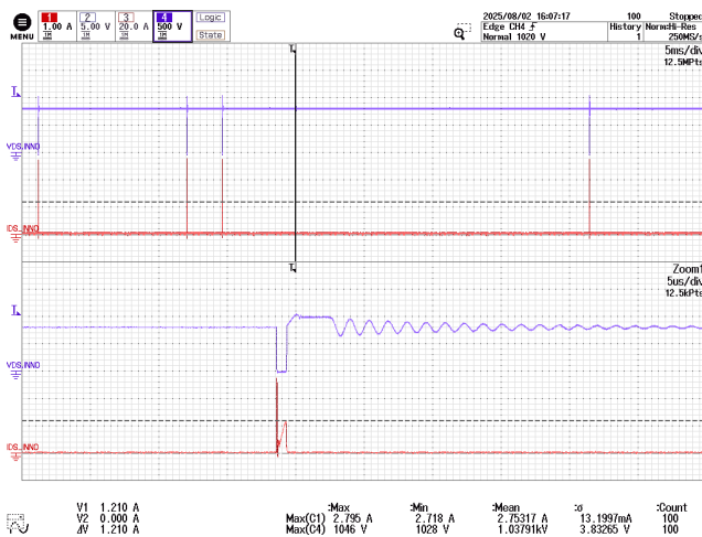
Figure 143 – InnoSwitch3-AQ Drain Voltage and Current. 800 VDC, No Load, 25 °C Ambient.
