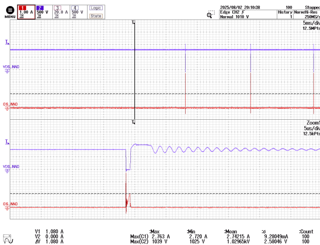
Figure 175 – InnoSwitch3-AQ Drain Voltage and Current. 800 VDC, No Load, -40 °C Ambient.
