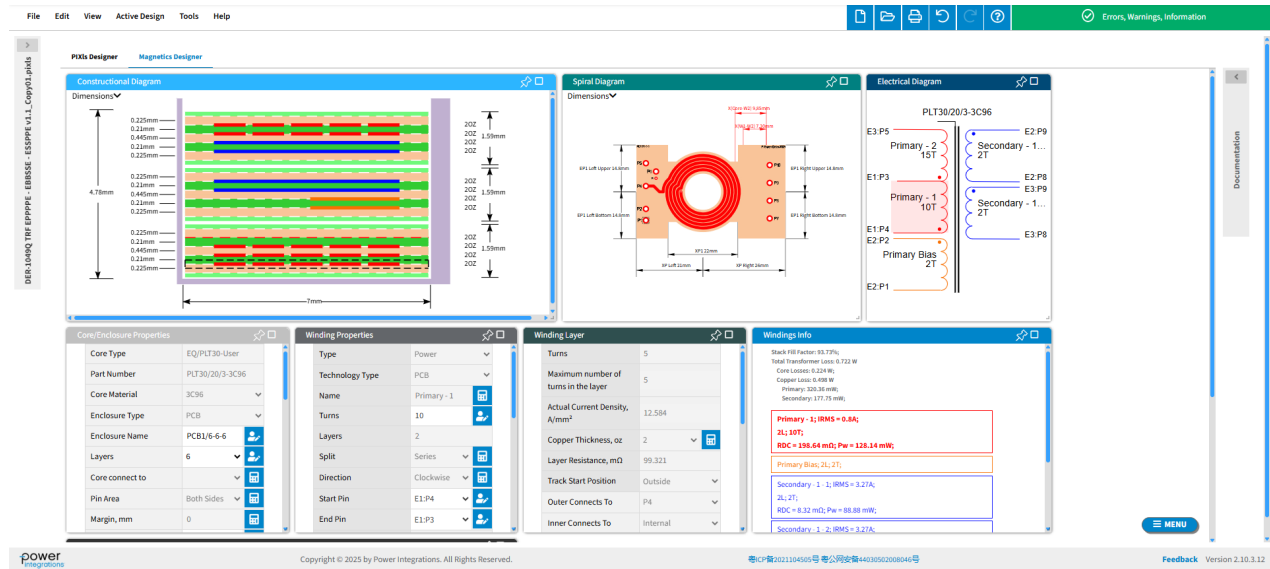
Figure 12 – PI Expert Online Magnetics Designer for Planar Transformer.
