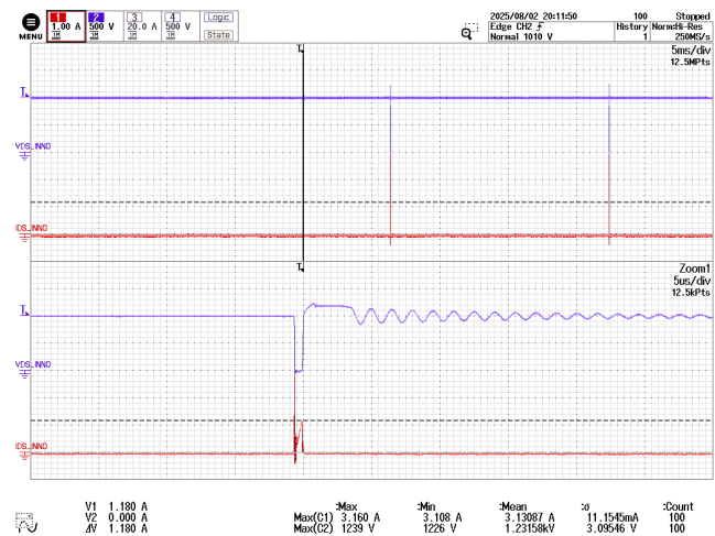
Figure 176 – InnoSwitch3-AQ Drain Voltage and Current. 1000 VDC, No Load, -40 °C Ambient.
