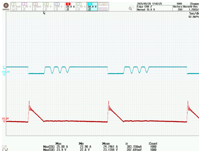
Figure 129 – SR FET Drain Voltage and Current. 80 VDC, 1.8 A Load, 85 °C Ambient. CH6: I_{D(SR)} , 20 A / div. CH8: V_{DS(SR)} , 50 V / div. Time: 5 \mu s / div.
