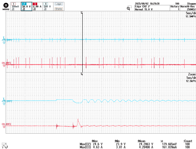
Figure 145 – SR FET Drain Voltage and Current. 80 VDC, No Load, 25 °C Ambient. CH2: V_{DS(SR)} , 50 V / div. CH3: I_{D(SR)} , 4 A / div. Time: 5 ms / div.
