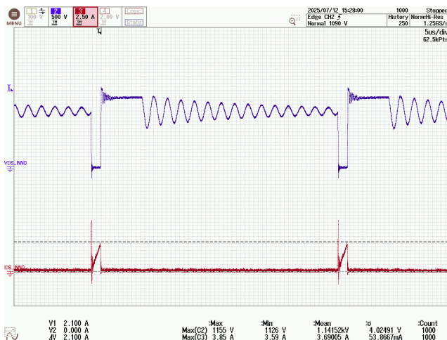
Figure 183 – InnoSwitch3-AQ Drain Voltage and Current. 800 VDC, 1.8 A Load, -40 °C Ambient. CH2: V_{DS(IC1)} , 500 V / div. CH3: I_{D(IC1)} , 2.5 A / div. Time: 5 \mu s / div.
