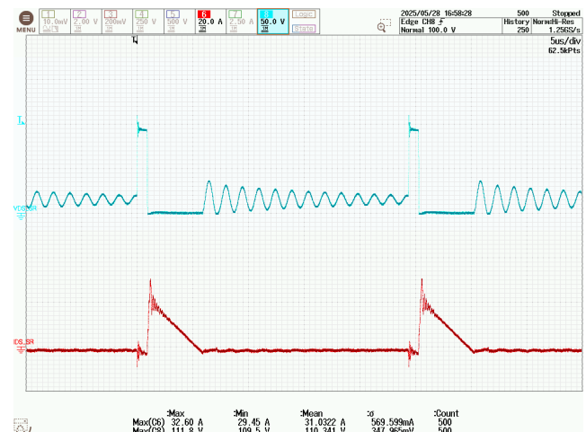
Figure 140 – SR FET Drain Voltage and Current. 1000 VDC, 2.33 A Load, 85 °C Ambient. CH6: I_{D(SR)} , 20 A / div. CH8: V_{DS(SR)} , 50 V / div. Time: 5 \mu s / div.
