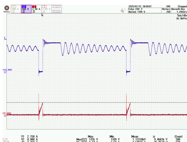
Figure 135 – InnoSwitch3-AQ Drain Voltage and Current. 800 VDC, 2.33 A Load, 85 °C Ambient.
