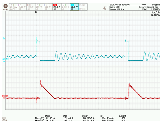
Figure 187 – SR FET Drain Voltage and Current. 800 VDC, 1.8 A Load, -40 °C Ambient.
