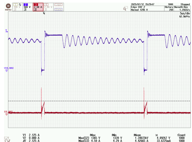
Figure 184 – InnoSwitch3-AQ Drain Voltage and Current. 1000 VDC, 1.8 A Load, -40 °C Ambient. CH2: V_{DS(IC1)} , 500 V / div. CH3: I_{D(IC1)} , 2.5 A / div. Time: 5 \mu s / div.
