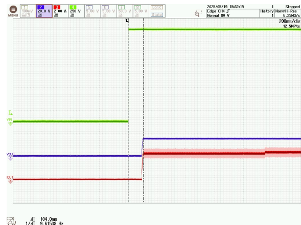
Figure 44 – Output Voltage and Current. 1000 VDC, 6.43 \Omega Load. CH2: V OUT , 20 V / div. CH3: I OUT , 2 A / div. CH4: V IN , 250 V / div. Time: 200 ms / div.
