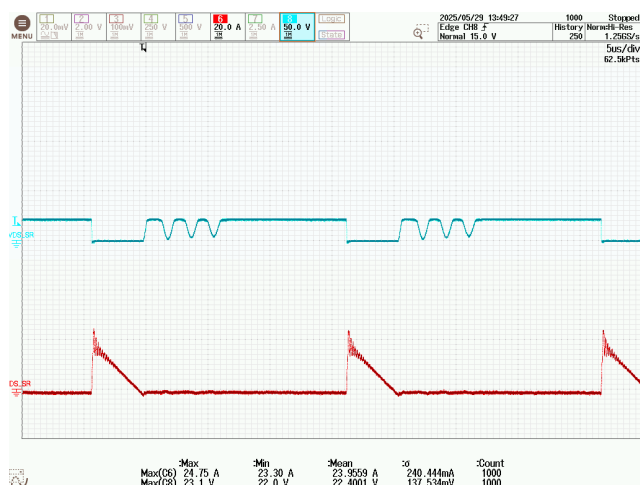
Figure 185 – SR FET Drain Voltage and Current. 80 VDC, 1.8 A Load, -40 °C Ambient.
