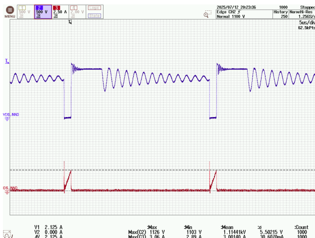
Figure 163 – InnoSwitch3-AQ Drain Voltage and Current. 800 VDC, 2.33 A Load, 25 °C Ambient.
