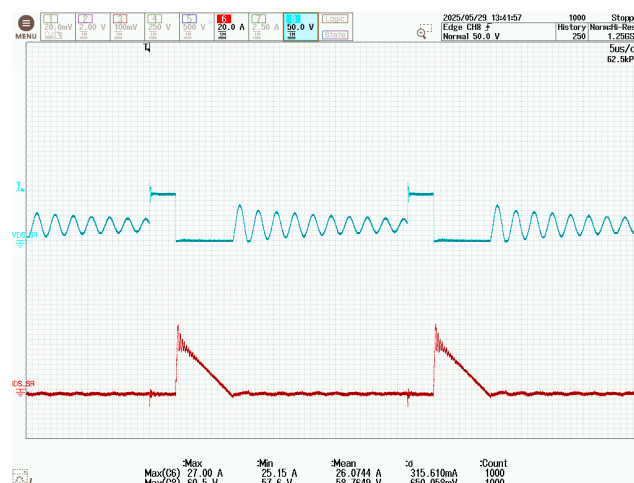
Figure 194 – SR FET Drain Voltage and Current. 400 VDC, 2.33 A Load, -40 °C Ambient. CH6: I_{D(SR)} , 20 A / div. CH8: V_{DS(SR)} , 50 V / div. Time: 5 \mu s / div.
