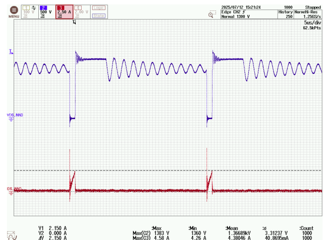
Figure 192 – InnoSwitch3-AQ Drain Voltage and Current. 1000 VDC, 2.33 A Load, -40 °C Ambient. CH2: V_{DS(IC1)} , 500 V / div. CH3: I_{D(IC1)} , 2.5 A / div. Time: 5 \mu s / div.
