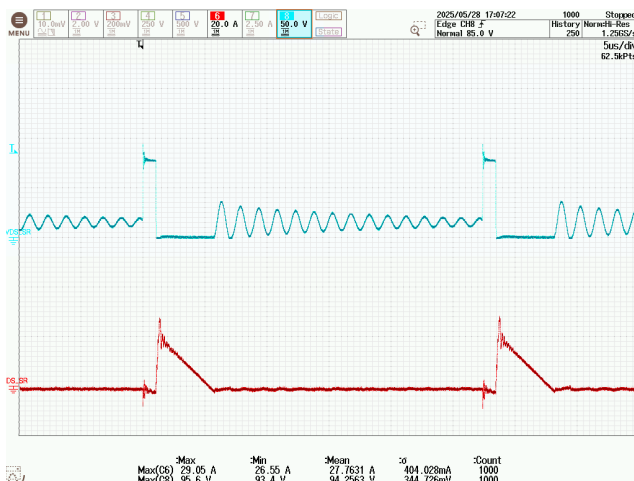
Figure 131 – SR FET Drain Voltage and Current. 800 VDC, 1.8 A Load, 85 °C Ambient. CH6: I_{D(SR)} , 20 A / div. CH8: V_{DS(SR)} , 50 V / div. Time: 5 \mu s / div.
