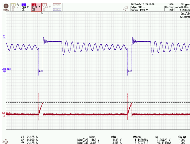
Figure 191 – InnoSwitch3-AQ Drain Voltage and Current. 800 VDC, 2.33 A Load, -40 °C Ambient. CH2: V_{DS(IC1)} , 500 V / div. CH3: I_{D(IC1)} , 2.5 A / div. Time: 5 \mu s / div.
