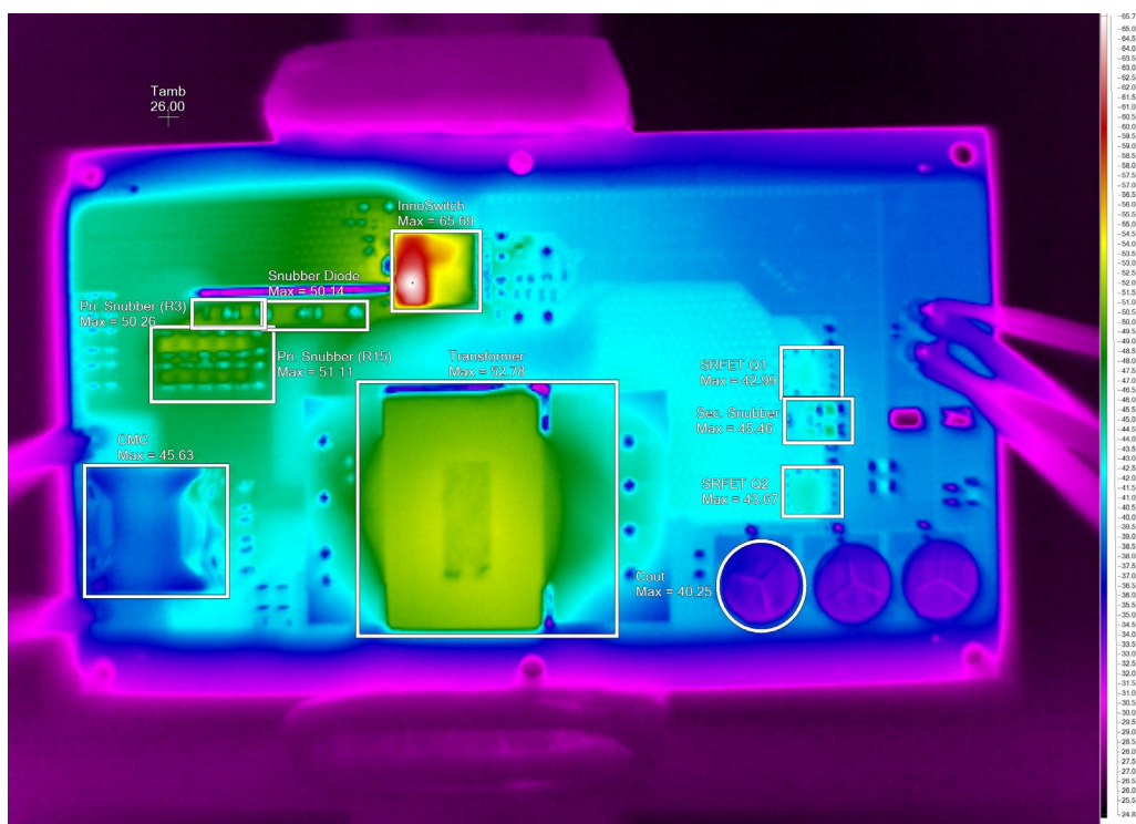
Figure 34 – Thermal Scan of the Top of the PCB at 800 V Input.
