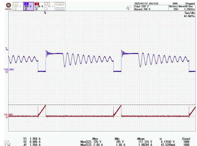
Figure 162 – InnoSwitch3-AQ Drain Voltage and Current. 400 VDC, 2.33 A Load, 25 °C Ambient.
