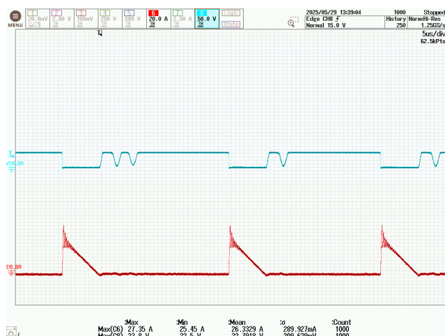
Figure 193 – SR FET Drain Voltage and Current. 80 VDC, 2.33 A Load, -40 °C Ambient. CH6: I_{D(SR)} , 20 A / div. CH8: V_{DS(SR)} , 50 V / div. Time: 5 \mu s / div.
