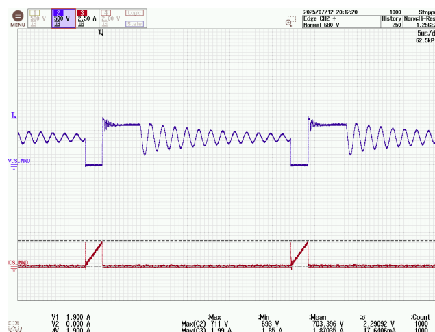
Figure 150 – InnoSwitch3-AQ Drain Voltage and Current. 400 VDC, 1.8 A Load, 25 °C Ambient.
