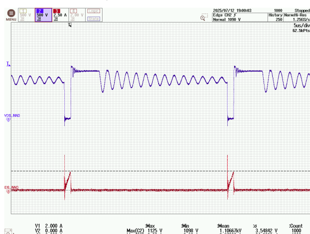
Figure 127 – InnoSwitch3-AQ Drain Voltage and Current. 800 VDC, 1.8 A Load, 85 °C Ambient.
