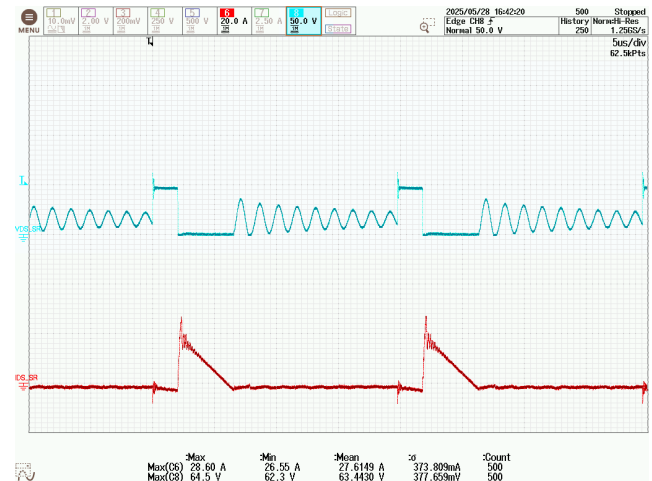
Figure 138 – SR FET Drain Voltage and Current. 400 VDC, 2.33 A Load, 85 °C Ambient. CH6: I_{D(SR)} , 20 A / div. CH8: V_{DS(SR)} , 50 V / div. Time: 5 \mu s / div.
