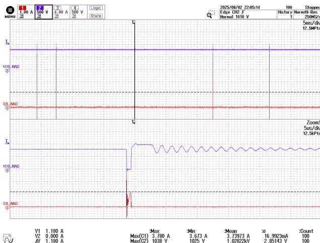
Figure 119 – InnoSwitch3-AQ Drain Voltage and Current. 800 VDC, No Load, 85 °C Ambient.
