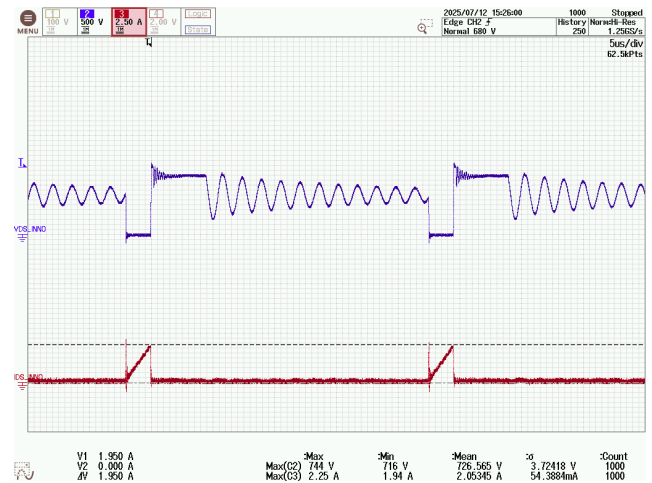
Figure 182 – InnoSwitch3-AQ Drain Voltage and Current. 400 VDC, 1.8 A Load, -40 °C Ambient. CH2: V_{DS(IC1)} , 500 V / div. CH3: I_{D(IC1)} , 2.5 A / div. Time: 5 \mu s / div.
