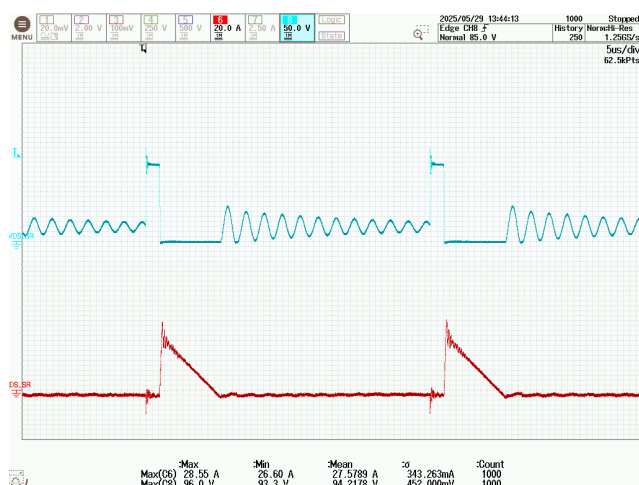
Figure 195 – SR FET Drain Voltage and Current. 800 VDC, 2.33 A Load, -40 °C Ambient. CH6: I_{D(SR)} , 20 A / div. CH8: V_{DS(SR)} , 50 V / div. Time: 5 \mu s / div.
