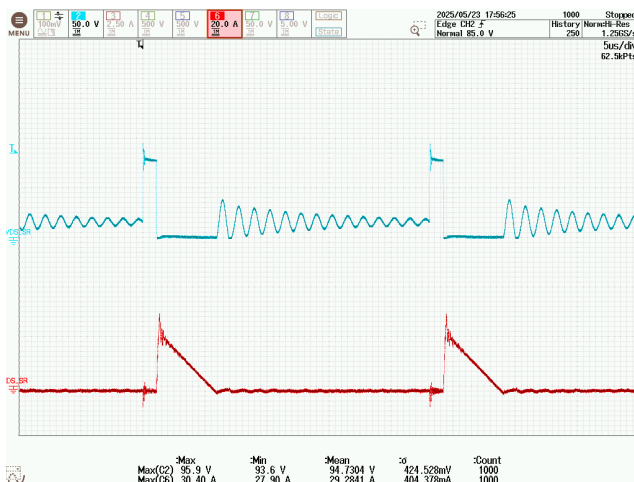
Figure 167 – SR FET Drain Voltage and Current. 800 VDC, 2.33 A Load, 25 °C Ambient. CH2: V_{DS(SR)} , 50 V / div. CH6: I_{D(SR)} , 20 A / div. Time: 5 \mu s / div.
