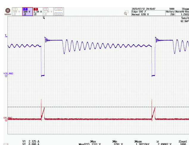
Figure 152 – InnoSwitch3-AQ Drain Voltage and Current. 1000 VDC, 1.8 A Load, 25 °C Ambient.
