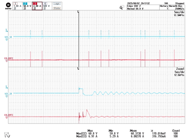
Figure 178 – SR FET Drain Voltage and Current. 400 VDC, No Load, -40 °C Ambient. CH2: V_{DS(SR)} , 50 V / div. CH3: I_{D(SR)} , 4 A / div. Time: 5 ms / div.
