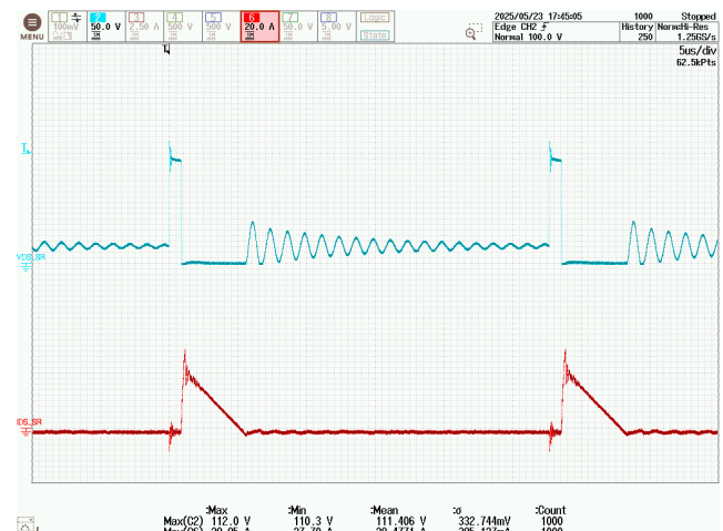
Figure 156 – SR FET Drain Voltage and Current. 1000 VDC, 1.8 A Load, 25 °C Ambient. CH2: V_{DS(SR)} , 50 V / div. CH6: I_{D(SR)} , 20 A / div. Time: 5 \mu s / div.
