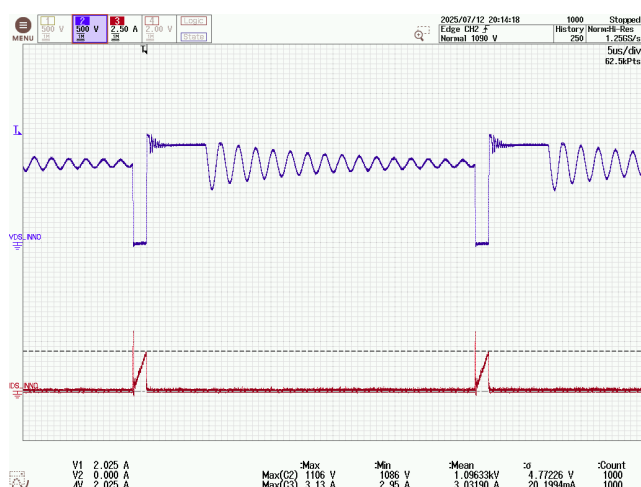
Figure 151 – InnoSwitch3-AQ Drain Voltage and Current. 800 VDC, 1.8 A Load, 25 °C Ambient.
