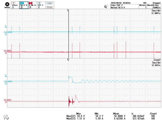
Figure 146 – SR FET Drain Voltage and Current. 400 VDC, No Load, 25 °C Ambient. CH2: V_{DS(SR)} , 50 V / div. CH3: I_{D(SR)} , 4 A / div. Time: 5 ms / div.
