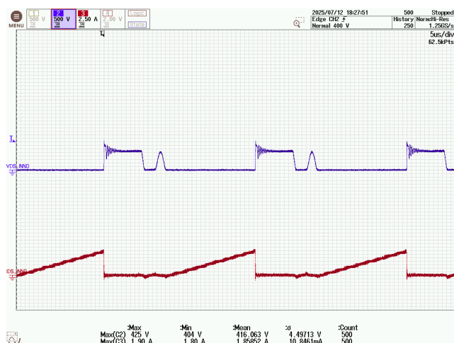
Figure 133 – InnoSwitch3-AQ Drain Voltage and Current. 80 VDC, 2.33 A Load, 85 °C Ambient.
