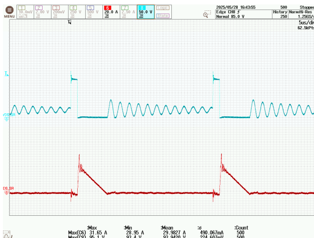
Figure 139 – SR FET Drain Voltage and Current. 800 VDC, 2.33 A Load, 85 °C Ambient. CH6: I_{D(SR)} , 20 A / div. CH8: V_{DS(SR)} , 50 V / div. Time: 5 \mu s / div.
