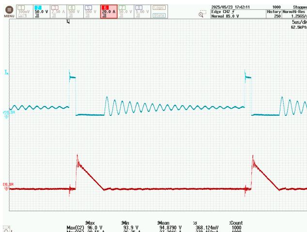
Figure 155 – SR FET Drain Voltage and Current. 800 VDC, 1.8 A Load, 25 °C Ambient. CH2: V_{DS(SR)} , 50 V / div. CH6: I_{D(SR)} , 20 A / div. Time: 5 \mu s / div.
