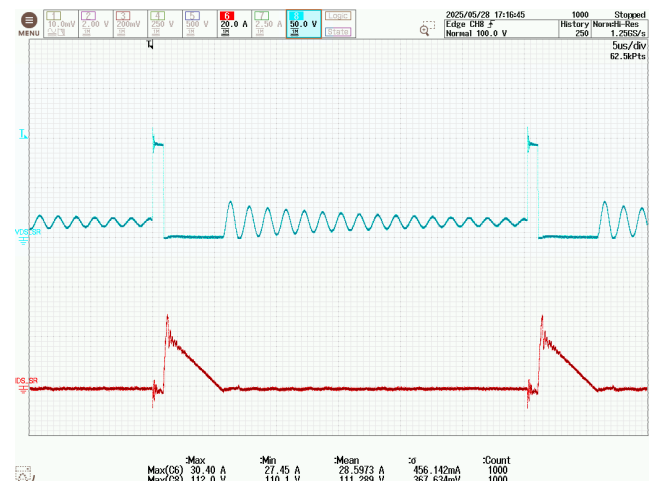
Figure 132 – SR FET Drain Voltage and Current. 1000 VDC, 1.8 A Load, 85 °C Ambient. CH6: I_{D(SR)} , 20 A / div. CH8: V_{DS(SR)} , 50 V / div. Time: 5 \mu s / div.
