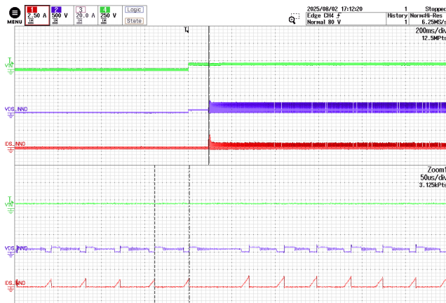
Figure 45 – INN3949CQ Drain Voltage and Current. 80 VDC, No Load.
