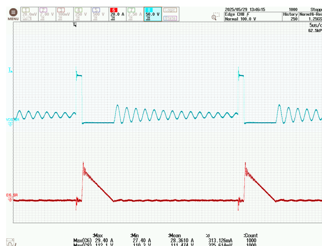
Figure 196 – SR FET Drain Voltage and Current. 1000 VDC, 2.33 A Load, -40 °C Ambient. CH6: I_{D(SR)} , 20 A / div. CH8: V_{DS(SR)} , 50 V / div. Time: 5 \mu s / div.
