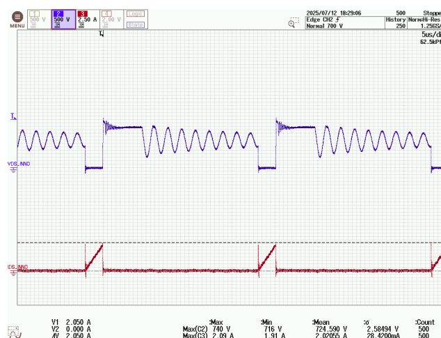
Figure 134 – InnoSwitch3-AQ Drain Voltage and Current. 400 VDC, 2.33 A Load, 85 °C Ambient.
