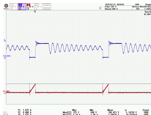
Figure 126 – InnoSwitch3-AQ Drain Voltage and Current. 400 VDC, 1.8 A Load, 85 °C Ambient.
