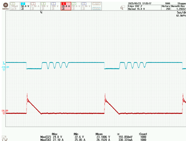
Figure 153 – SR FET Drain Voltage and Current. 80 VDC, 1.8 A Load, 25 °C Ambient. CH2: V_{DS(SR)} , 50 V / div. CH6: I_{D(SR)} , 20 A / div. Time: 5 \mu s / div.
