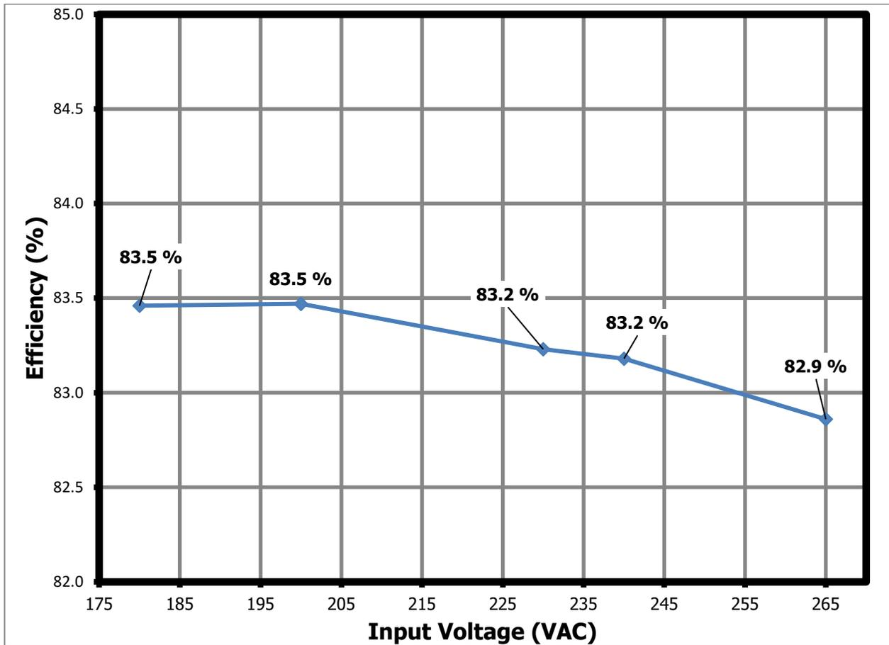
Figure 21 – Efficiency vs. Input Line Voltage, SVF Enabled.
