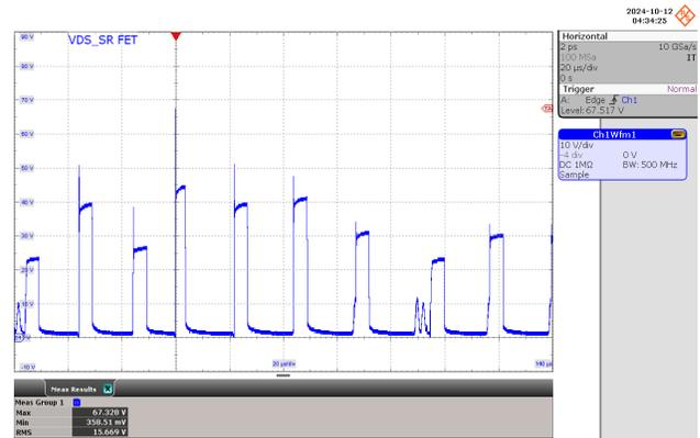
**Figure 70** – SR FET Drain Voltage
