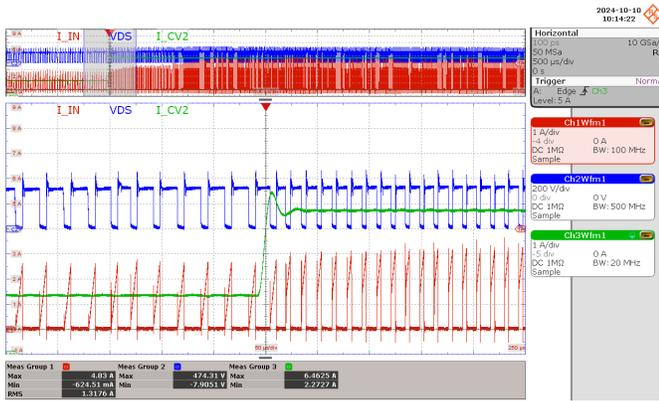
**Figure 63** – CV2 Output-Load Transient at 180 VAC;
