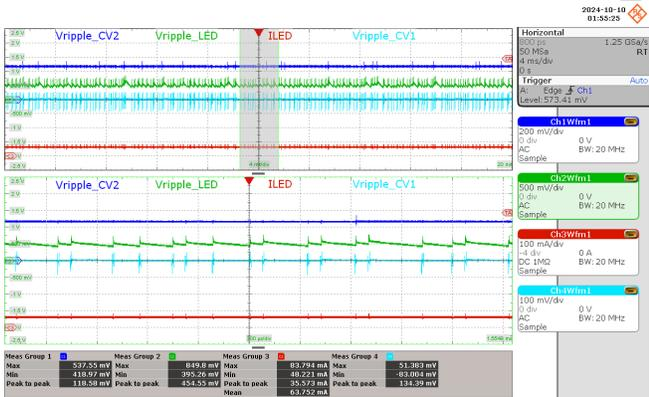
**Figure 84** – Output Ripple Voltage
