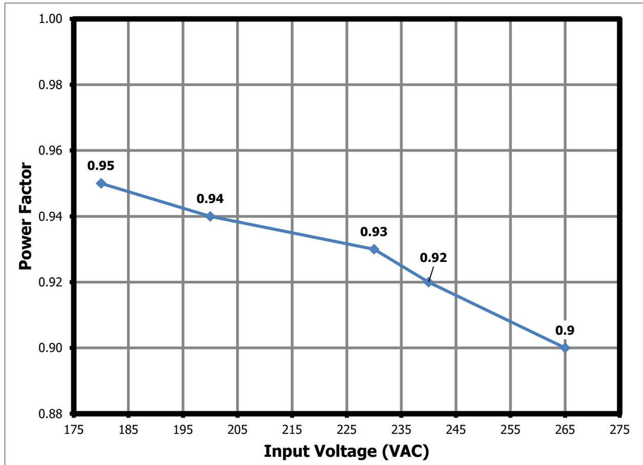
**Figure 23** – Power Factor vs Input Line, SVF Enabled, P<sub>OUT</sub> = 24.1 W.
