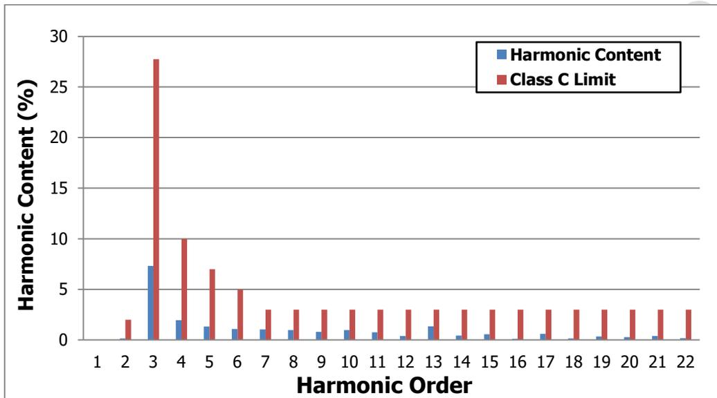
Figure 32 – Harmonic Content, SVF Enabled, P<sub>OUT</sub> = 24.1 W, Test 1, 230 VAC.
