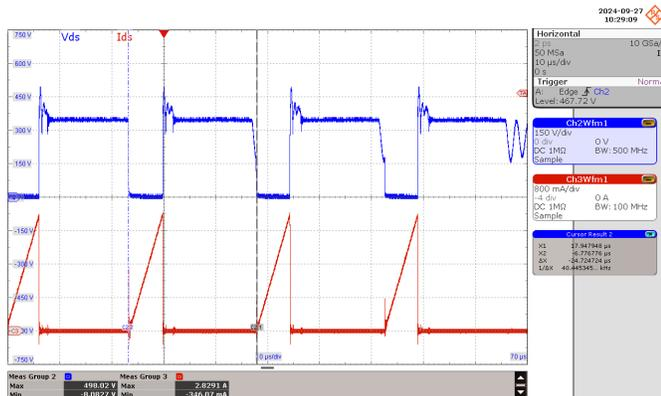
**Figure 60** – Primary Drain Voltage and Current
