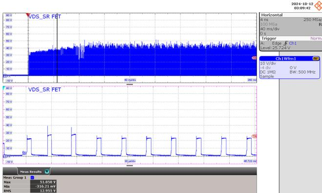
**Figure 66** – SR FET Drain Voltage
