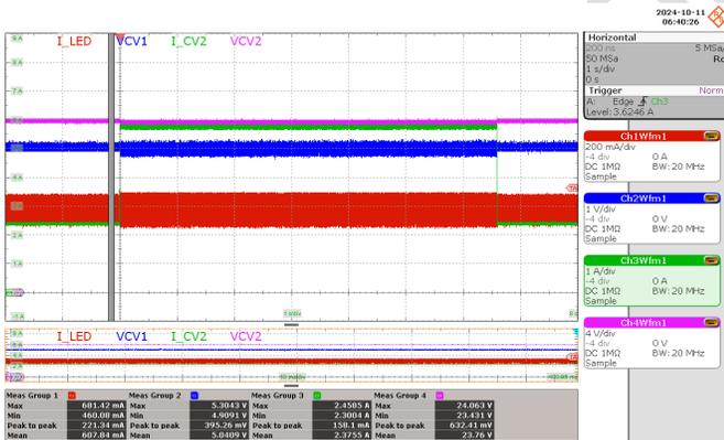
**Figure 74** – Load Transient during Nominal Load at 230 VAC, LED: 36 V / 0.6 A, CV2: 24 V / 2.4 A – 5.8 A Transient, CV1: 5 V / 0.5 A,
