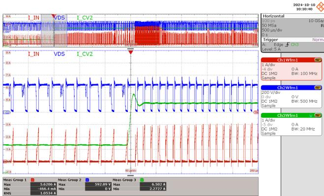
**Figure 65**– CV2 Output-Load Transient at 265 VAC;
