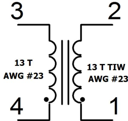
Figure 16 – Inductor Electrical Diagram.
