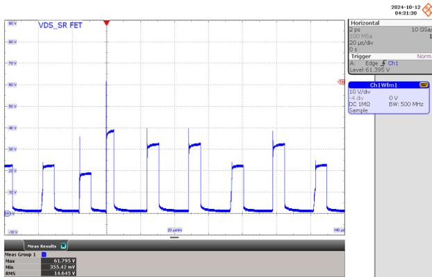
**Figure 69** – SR FET Drain Voltage
