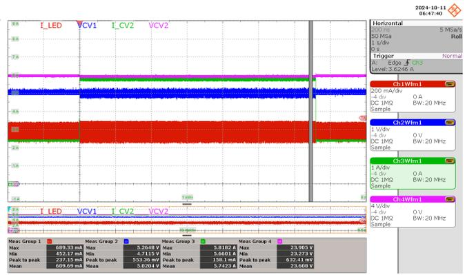
**Figure 75** – Load Transient during Peak Load at 230 VAC, LED: 36 V / 0.6 A, CV2: 24 V / 2.4 A – 5.8 A Transient, CV1: 5 V / 0.5 A,
