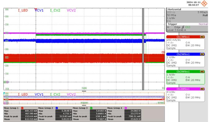
**Figure 73** – Load Transient during Peak Load at 180 VAC, LED: 36 V / 0.6 A, CV2: 24 V / 2.4 A – 5.8 A Transient, CV1: 5 V / 0.5 A,
