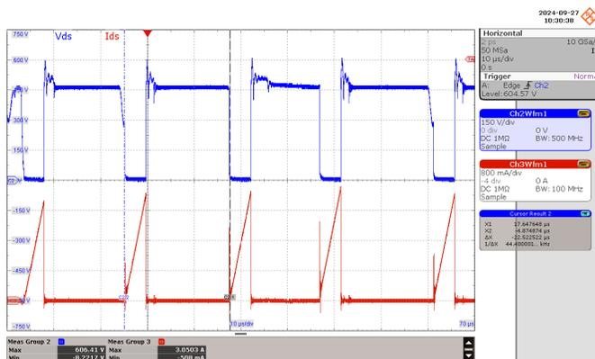
**Figure 62** – Primary Drain Voltage and Current
