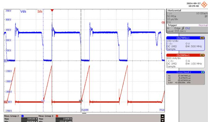
**Figure 61** – Primary Drain Voltage and Current
