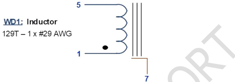
Figure 12 – Electrical Diagram.
