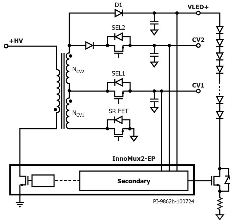
**Figure 3** – DER-1050 Block Diagram of Secondary Side.
