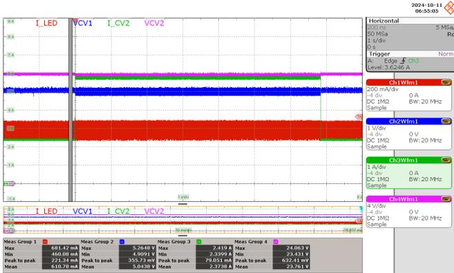
**Figure 72** – Load Transient during Nominal Load at 180 VAC, LED: 36 V / 0.6 A, CV2: 24 V / 2.4 A – 5.8 A Transient, CV1: 5 V / 0.5 A,
