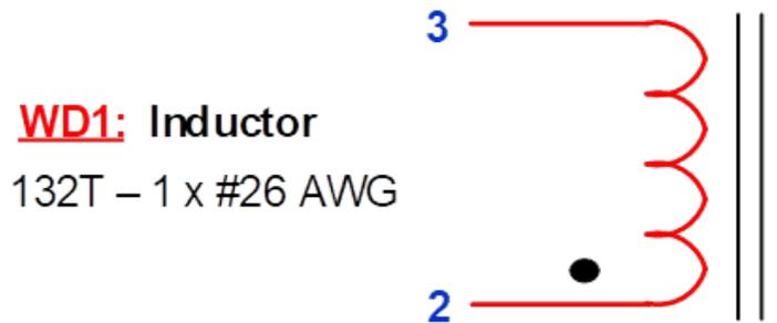
Figure 14 – Electrical Diagram.
