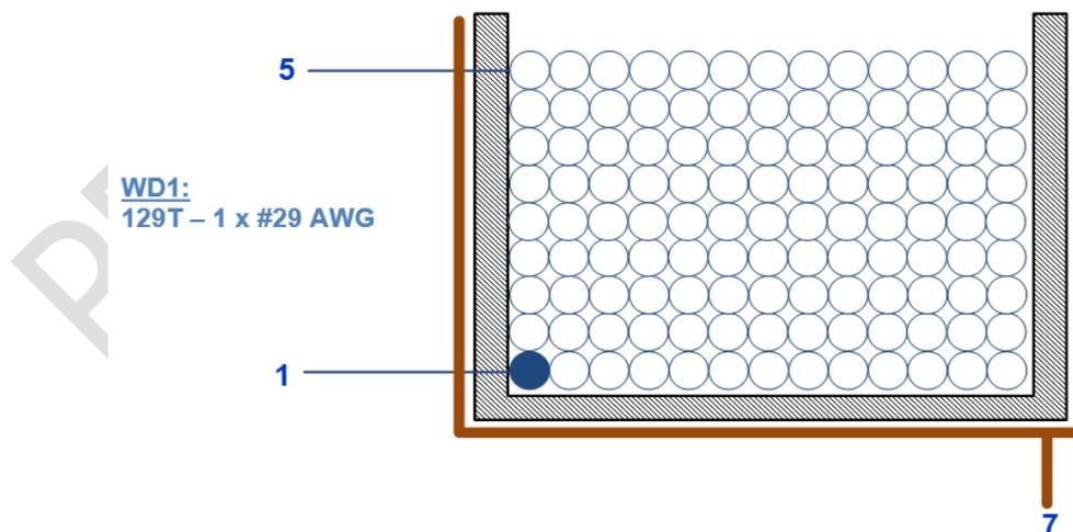
Figure 13 – Inductor Build Diagram.
