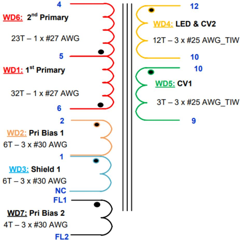
Figure 10 – Transformer Schematic.
