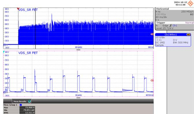
**Figure 67** – SR FET Drain Voltage
