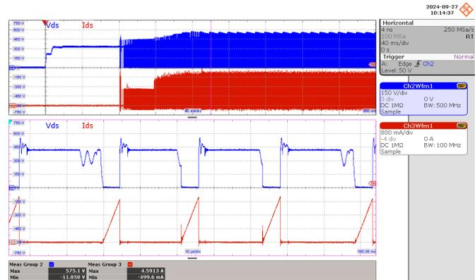
**Figure 58** – Primary Drain Voltage and Current
