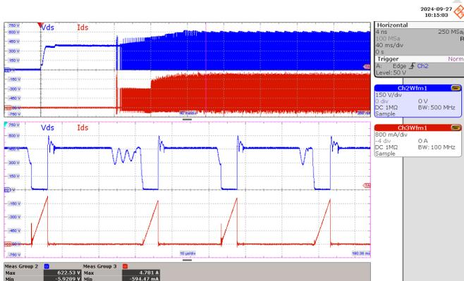
**Figure 59** – Primary Drain Voltage and Current
