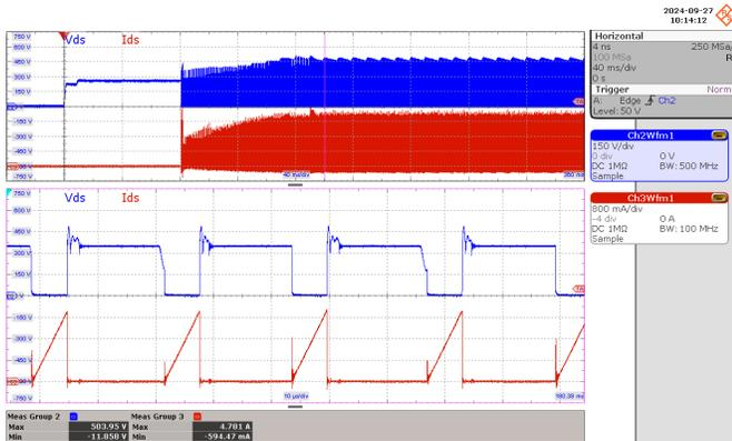
**Figure 57** – Primary Drain Voltage and Current
