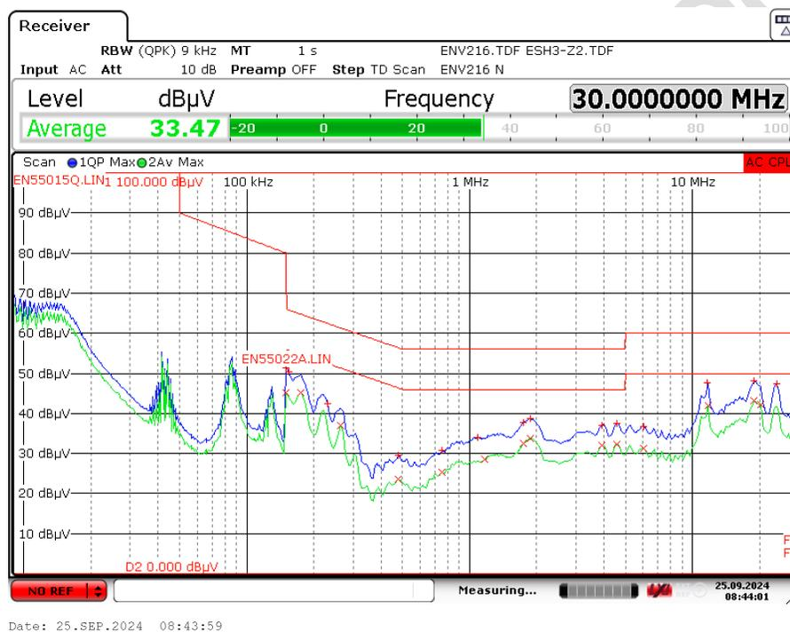
**Figure 85** – Conducted EMI with SVF Disabled, Full Load, 230 VAC.
