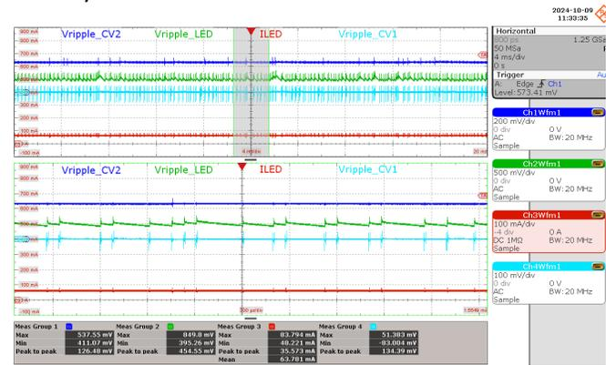
**Figure 82** – Output Ripple Voltage
