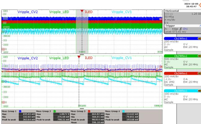
**Figure 81** – Output Ripple Voltage
