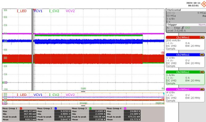
**Figure 76** – Load Transient during Nominal Load at 265 VAC, LED: 36 V / 0.6 A, CV2: 24 V / 2.4 A – 5.8 A Transient, CV1: 5 V / 0.5 A,
