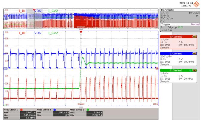
**Figure 64** – CV2 Output-Load Transient 230 VAC;
