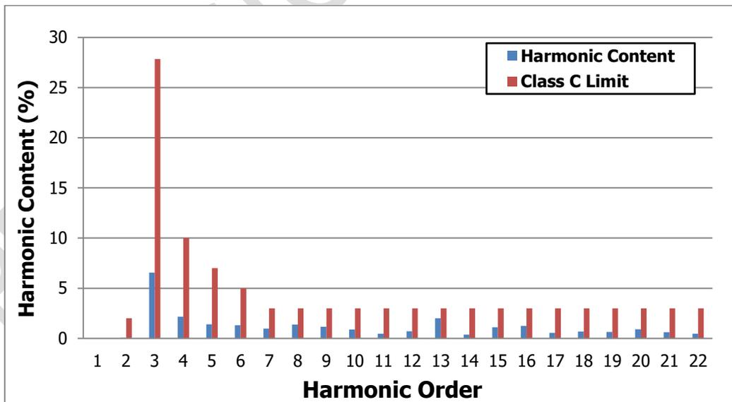
Figure 33 – Harmonic Content, SVF Enabled, P<sub>OUT</sub> = 21.6 W, Test 2, 230 VAC.
