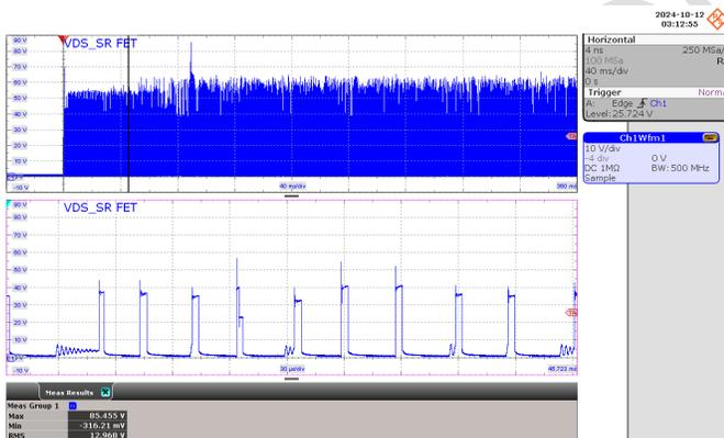
**Figure 68** – SR FET Drain Voltage
