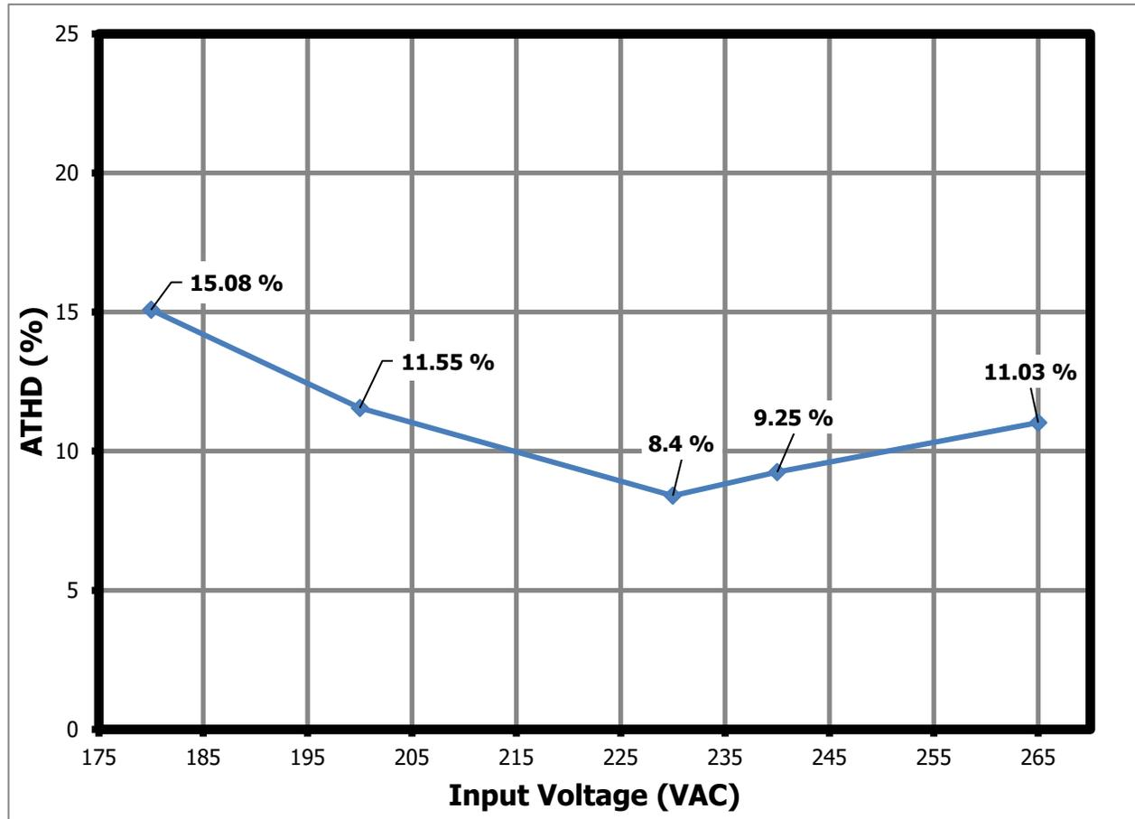
Figure 24 – THD vs Input Line, SVF Enabled, P<sub>OUT</sub> = 24.1 W.
