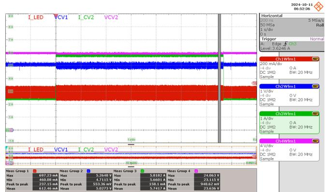
**Figure 77** – Load Transient during Peak Load at 265 VAC, LED: 36 V / 0.6 A, CV2: 24 V / 2.4 A – 5.8 A Transient, CV1: 5 V / 0.5 A,
