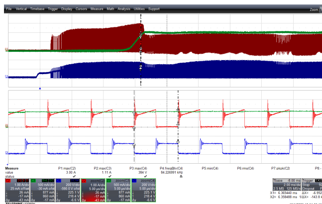
Figure 65 – 120 VAC, 60 Hz. 36 V LED String.
