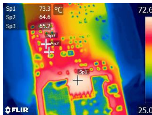
Figure 29 – Thermal Scan 120 V 36 V / 1 A Sp1: U2-(TNY5075K): 73.3 °C Sp2: D8-(Snubber Diode): 64.6 °C Sp3: D7-(Snubber Diode): 65.2 °C
