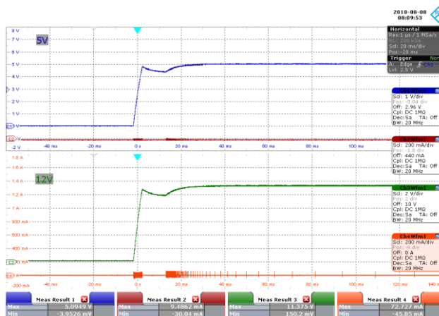
Figure 40 – 115 VAC 60 Hz, No-Load Start-up. CH1: 5 V OUT , 1 V / div., 20 ms / div. CH2: 5 V I LOAD , 200 mA / div., 20 ms / div. CH3: 12 V OUT , 2 V / div., 20 ms / div. CH4: 12 V I LOAD , 200 mA / div., 20 ms / div.
