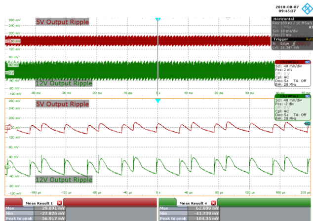
Figure 98 – 85 VAC 60 Hz, 100% Load. CH2: 5 V OUT , 40 mV / div., 10 ms / div. CH3: 12 V OUT , 40 mV / div., 10 ms / div. Zoom: 40 μs / div. 5 V Output Ripple = 55.536 mV. 12 V Output Ripple = 112.25 mV.
