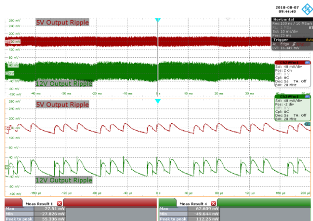
Figure 98 – 85 VAC 60 Hz, 100% Load. CH2: 5 V OUT , 40 mV / div., 10 ms / div. CH3: 12 V OUT , 40 mV / div., 10 ms / div. Zoom: 40 μs / div. 5 V Output Ripple = 55.536 mV. 12 V Output Ripple = 112.25 mV.
