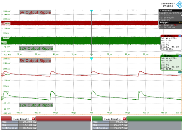
Figure 110 – 85 VAC 60 Hz, 25% Load. CH2: 5 V OUT , 40 mV / div., 10 ms / div. CH3: 12 V OUT , 40 mV / div., 10 ms / div. Zoom: 40 μs / div. 5 V Output Ripple = 36.364 mV. 12 V Output Ripple = 69.565 mV.
