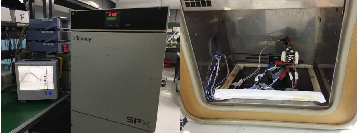
Figure 135 – Thermal Performance Set-up using Thermal Chamber.
