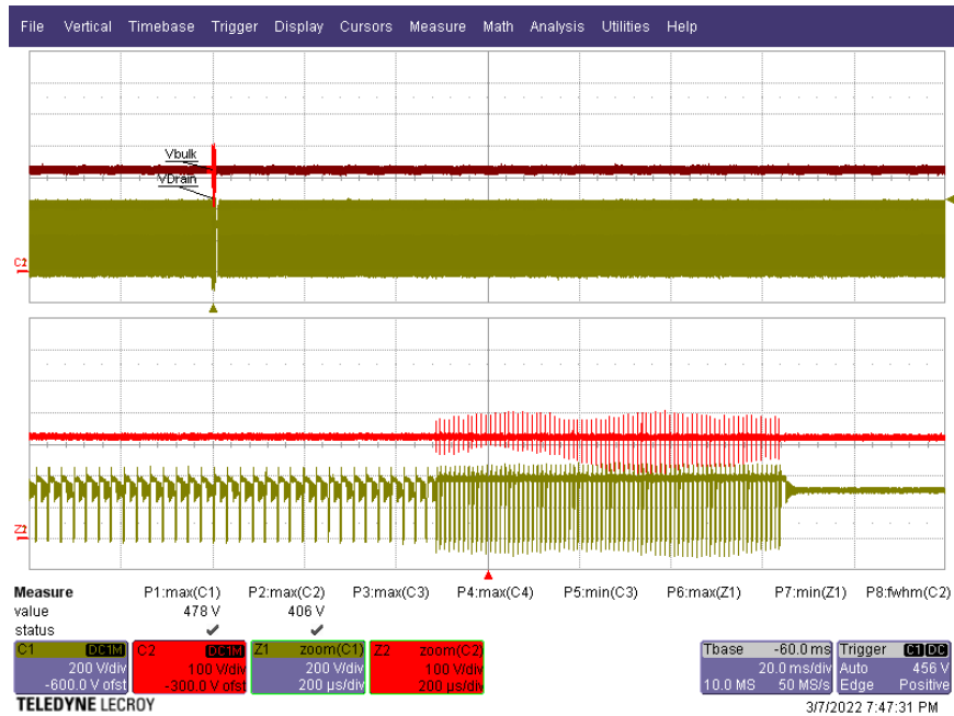
Figure 80 – 4 kV EFT Test. InnoSwitch3-TN V_{DS(MAX)} : 478, V_{BULK(MAX)} : 406 V. Upper: V_{BULK} , 200 V / div, 20 ms / div. Lower: InnoSwitch3-TN V_{DS} , 100 V / div, 20 ms / div. Zoom: 200 \mu s / div.
