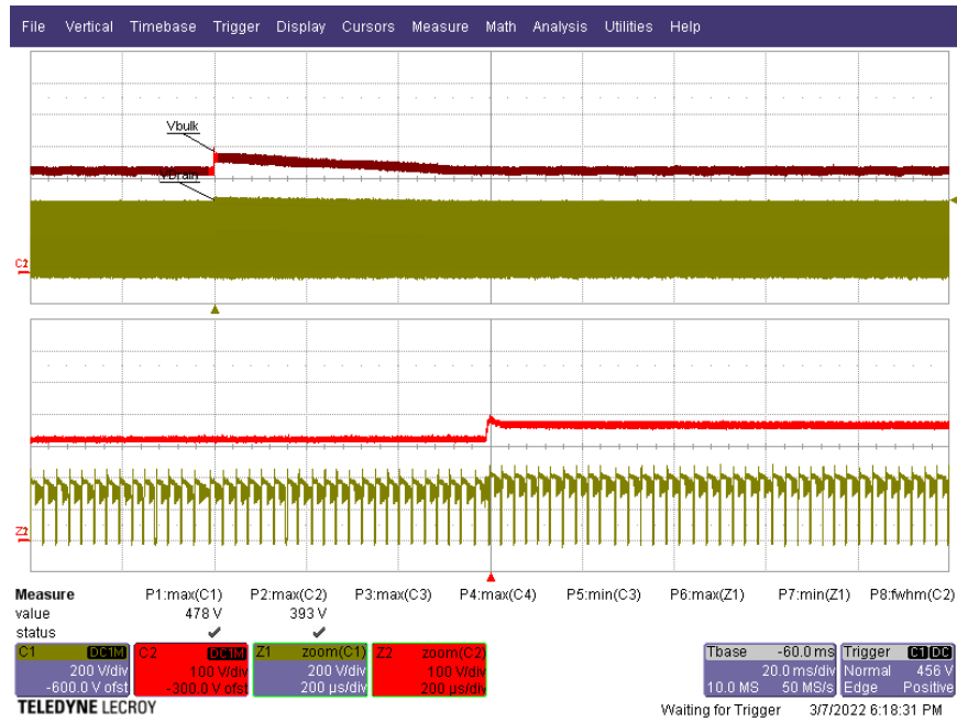
Figure 79 – 6 kV Ring Wave Test. InnoSwitch3-TN V_{DS(MAX)} : 478, V_{BULK(MAX)} : 393 V. Upper: V_{BULK} , 200 V / div, 20 ms / div. Lower: InnoSwitch3-TN V_{DS} , 100 V / div, 20 ms / div. Zoom: 200 \mu s / div.
