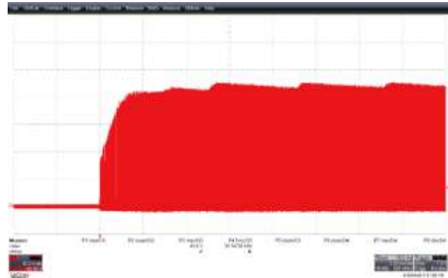
Figure 32 – SR FET Voltage Waveforms During Start-Up. 265 VAC Input, Full Load. (45.6V V MAX ) CH1: V DRAIN , 10 V / div, 5 ms / div.
