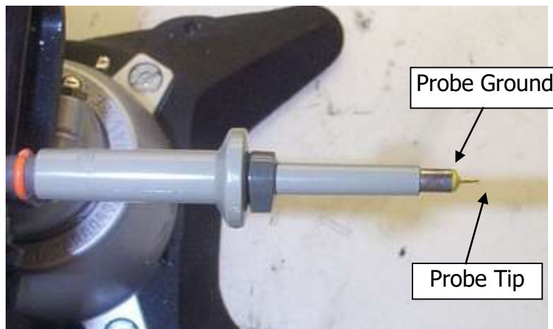
Figure 36 – Oscilloscope Probe Prepared for Ripple Measurement. (End Cap and Ground Lead Removed.)
