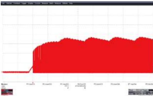
Figure 27 – Drain Voltage and Current Waveforms. 85 VAC Input, Full Load. CH1: V_{DRAIN} , 100 V / div, 5 ms / div.
