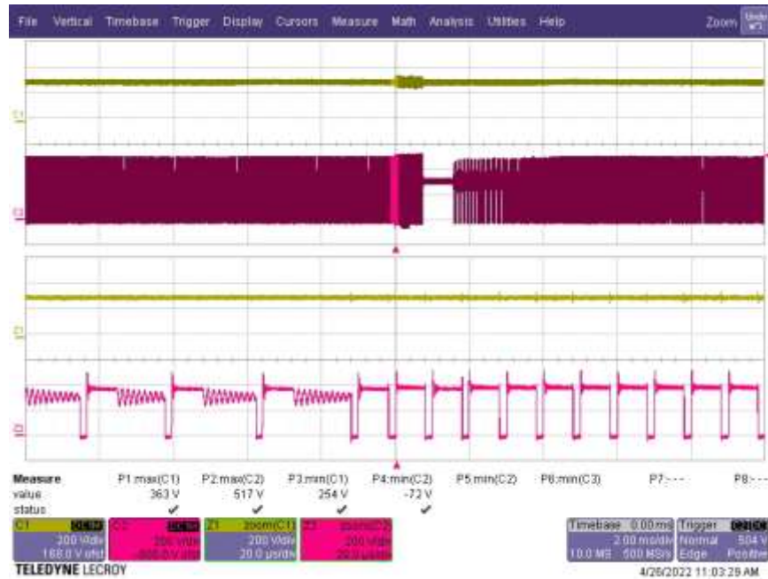
Figure 56 – 2 kV EFT Test. InnoSwitch3-TN V_{DS(MAX)} : 517 V, V_{BULK(MAX)} : 363 V. Upper: V_{BULK} , 200 V / div, 2 ms / div. Lower: InnoSwitch3-TN V_{DS} , 200 V / div, 2 ms / div. Zoom: 20 \mu s / div.
