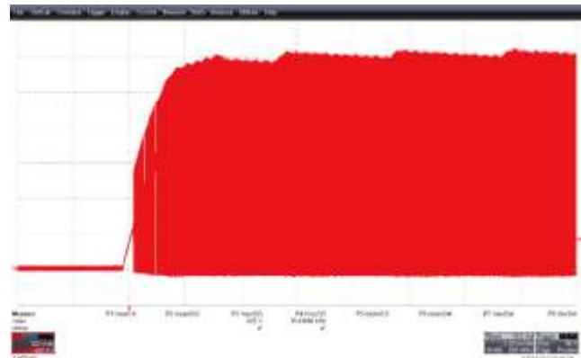
Figure 28 – Drain Voltage and Current Waveforms. 265 VAC Input, Full Load, (625 V_{MAX} ). CH1: V_{DRAIN} , 100 V / div, 5 ms / div.
