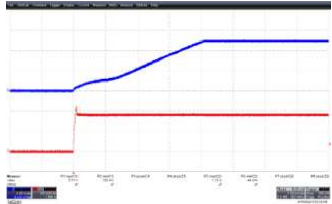
Figure 35 – Output Voltage and Current Waveforms. 265 VAC Input. Upper: 5 V OUT , 2 V / div. Lower: 5 I OUT , 500 mA / div. 2 ms / div.
