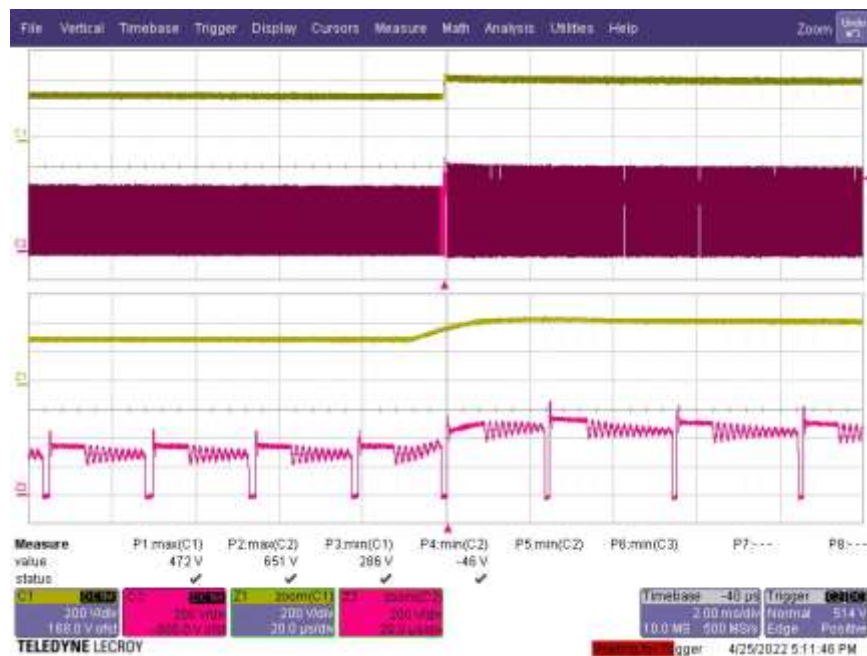
Figure 54 – 1 kV Differential Mode Surge Test. InnoSwitch3-TN V_{DS(MAX)} : 651 V, V_{BULK(MAX)} : 472 V. Upper: V_{BULK} , 200 V / div, 2 ms / div. Lower: InnoSwitch3-TN V_{DS} , 200 V / div, 2 ms / div. Zoom: 20 \mu s / div.
