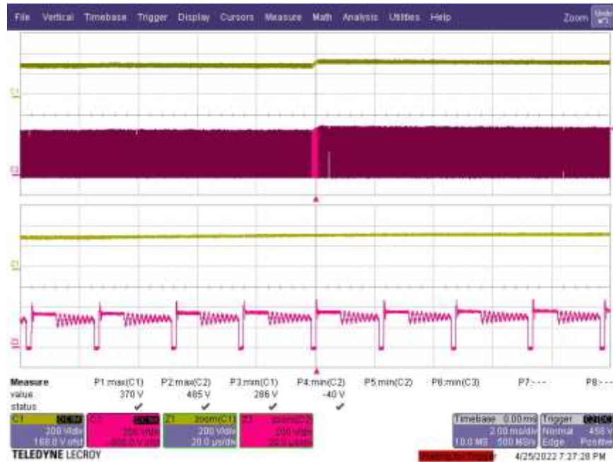
Figure 55 – 6 kV Ring Wave Test. InnoSwitch3-TN V_{DS(MAX)} : 485 V, V_{BULK(MAX)} : 370 V. Upper: V_{BULK} , 200 V / div, 2 ms / div. Lower: InnoSwitch3-TN V_{DS} , 200 V / div, 2 ms / div. Zoom: 20 \mu s / div.
