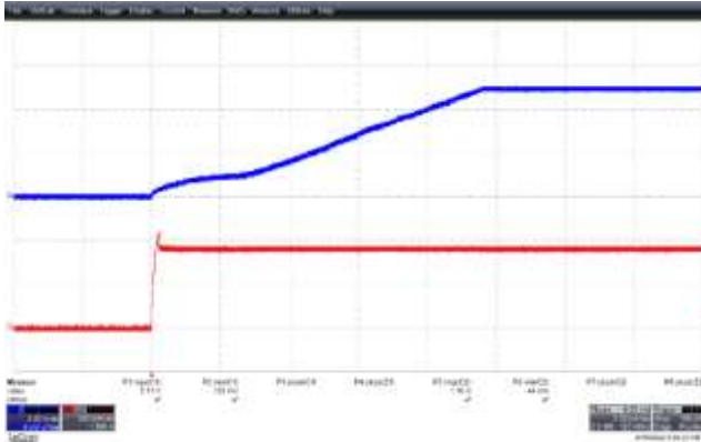
Figure 34 – Output Voltage and Current Waveforms. 85 VAC Input. Upper: 5 V OUT , 2 V / div. Lower: 5 I OUT , 500 mA / div. 2 ms / div.
