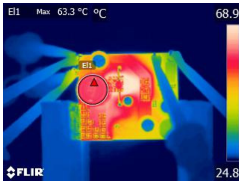
Figure 13 – Output Choke (E1), 63.3 °C. 85 VAC, 1 A Output.
