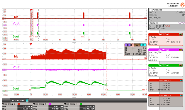
Figure 44 – Drain Current and Output Waveforms. 85 VAC Input. Drain Current: 2 A / div., 500 ms / div. Output Voltage: 500 mV / div., 500 ms / div. Output Current: 2 A / div., 500 ms / div. Zoom = 10 ms / div.
