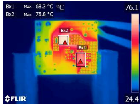
Figure 16 – LNK3209G (Bx1), 68.3 °C. Buck Diode (Bx2), 78.8 °C. 135 VAC, 1 A Output.
