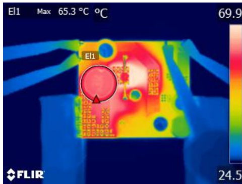
Figure 15 – Output Choke (E1), 65.3 °C. 135 VAC, 1 A Output.
