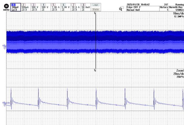
Figure 114 – Output Voltage Ripple. 200 VDC, 1.46 A Load, 85 °C Ambient. CH1: V_{OUT} , 100 mV / div. Time: 10 ms / div. V_{RIPPLE} = 340 mV.
