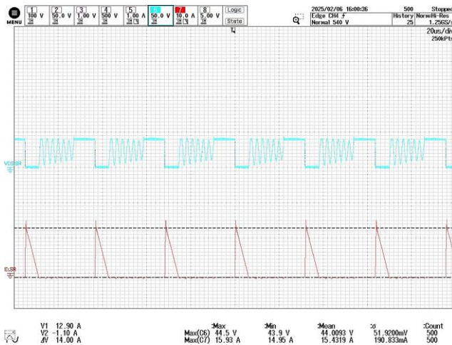
Figure 88 – SR FET Drain Voltage and Current. 200 VDC, 1.46 A Load, 25 °C Ambient. CH6: V_{DS,SRFET} , 50 V / div. CH7: I_{D,SRFET} , 10 A / div. Time: 20 \mu s / div.
