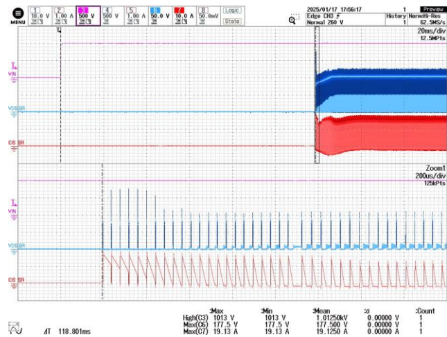
Figure 59 – SR FET Drain Voltage and Current. 1000 VDC, 16.3 Ω Load. CH3: V_{IN} , 500 V / div. CH6: V_{DS,SRFET} , 50 V / div. CH7: I_{D,SRFET} , 10 A / div. Time: 200 ms / div.
