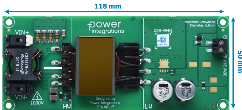
Figure 2 – Populated Circuit Board, Top.
