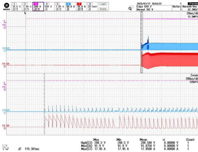
Figure 56 – SR FET Drain Voltage and Current. 200 VDC, 16.3 Ω Load. CH3: V_{IN} , 200 V / div. CH6: V_{DS,SRFET} , 50 V / div. CH7: I_{D,SRFET} , 10 A / div. Time: 200 ms / div.
