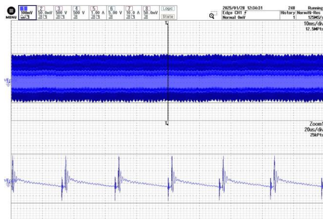
Figure 114 – Output Voltage Ripple. 200 VDC, 1.46 A Load, 85 °C Ambient. CH1: V_{OUT} , 100 mV / div. Time: 10 ms / div. V_{RIPPLE} = 340 mV.
