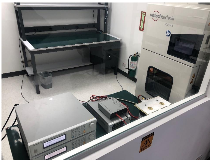
Figure 17 – Set-up for Test Inside the High-Voltage Room.
