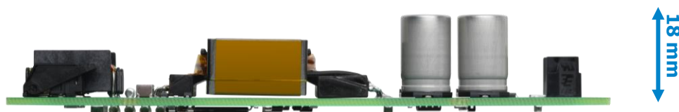
Figure 4 – Populated Circuit Board, Side.
