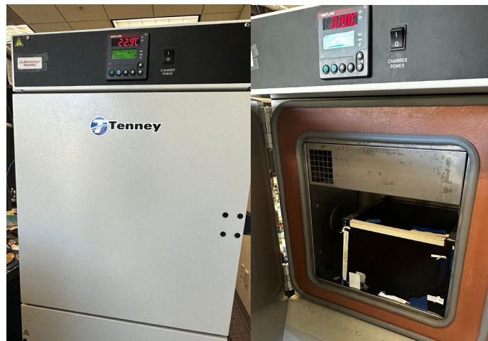
Figure 55 – Thermal Chamber Test Set-up.
