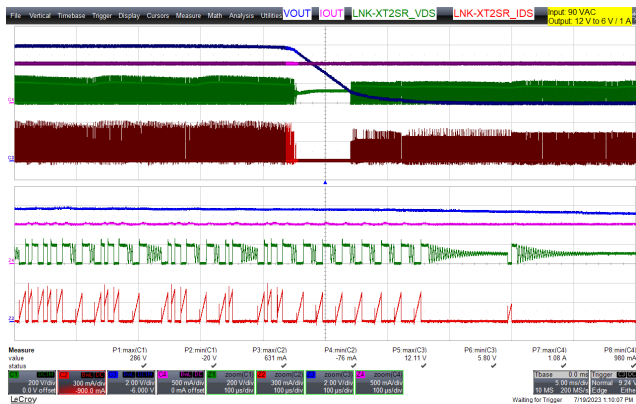
Figure 106 – Output Voltage Transient Waveforms. 90 VAC Input, Full Load. Upper: V OUT , 2 V / div. Upper Middle: I OUT , 500 mA / div. Lower Middle: LNK-XT2SR_V DS . 200 V / div. Lower: LNK-XT2SR_I DS , 300 mA / div. 5 ms / div. Zoom: 100 μs / div.
