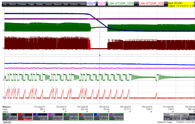
Figure 110 – Output Voltage Transient Waveforms. 90 VAC Input, Full Load. Upper: V_{OUT} , 2 V / div. Upper Middle: I_{OUT} , 100 mA / div. Lower Middle: LNK-XT2SR_ V_{DS} . 200 V / div. Lower: LNK-XT2SR_ I_{DS} , 300 mA / div. 100 ms / div. Zoom: 20 ms / div.
