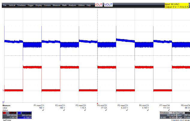
Figure 78 – 0 A – 1 A, 6 V Load Step Transient Response, 90 VAC. 6 V MAX : 6.23 V.; 6 V MIN : 5.75 V. Upper: 12 V OUT . 200 mV / div. Lower: 12 I OUT , 500 mA / div. 100 ms / div.
