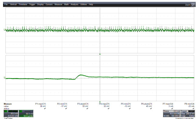
Figure 173 – Output Ripple Voltage Waveforms. 265 VAC Input. 6 V PK-PK : 55 mV. Upper: 6 V OUT , 50 mV / div, 10 ms / div. Zoom: 50 μs / div.
