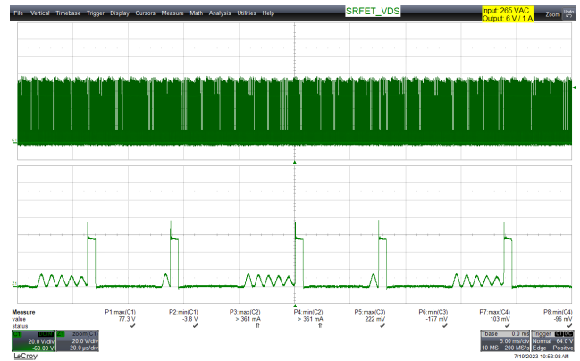
Figure 119 – SRFET Voltage Waveforms. 265 VAC Input, Full Load (77.3 V MAX ). Upper: SRFET_Vds. 20 V / div. 5 ms / div. Zoom: 20 us / div.
