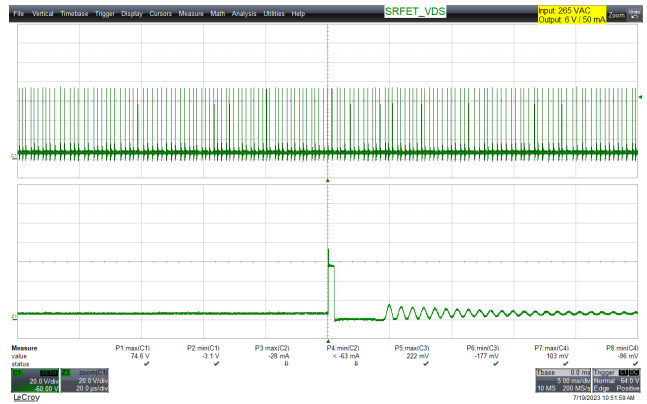
Figure 121 – SRFET Voltage Waveforms. 265 VAC Input, 50 mA Load (74.6 V MAX ). Upper: SRFET_Vds. 20 V / div. 5 ms / div. Zoom: 20 us / div.
