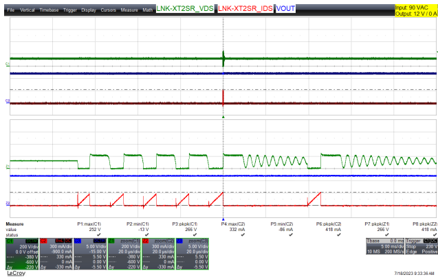
Figure 84 – Drain Voltage and Current Waveforms. 90 VAC Input, No-Load. Upper: LNK-XT2SR_V DS . 200 V / div. Middle: 12 V OUT , 5 V / div. Lower: LNK-XT2SR_I DS , 300 mA / div. 5 ms / div. Zoom: 20 μs / div.
