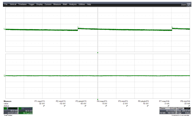
Figure 153 – Output Ripple Voltage Waveforms. 265 VAC Input. 6 V PK-PK : 43 mV. Upper: 6 V OUT , 50 mV / div, 10 ms / div. Zoom: 50 μs / div.
