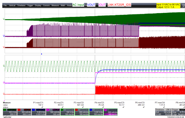
Figure 190 – Brown-In Waveforms. 0 to 90 VAC Input, Full Load. Upper: AC Input, 100 V / div. Upper Middle: 12 V OUT , 5 V / div. Lower Middle: 12 I OUT , 500 mA / div. Lower: LNK-XT2SR_I DS , 300 mA / div. 100 s / div. Zoom: 100 ms / div. Brown-In Voltage = 65.8 VAC
