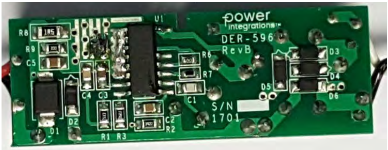
Figure 3 – Populated Circuit Board, Bottom View.
