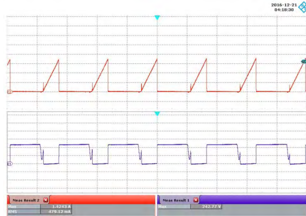
Figure 43 – 115 VAC, 80 V LED Load. Upper: I_{DRAIN} , 400 mA / div. Lower: V_{DRAIN} , 100 V / div., 5 \mu s / div.
