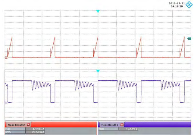
Figure 47 – 277 VAC, 80 V LED Load. Upper: I_{DRAIN} , 400 mA / div. Lower: V_{DRAIN} , 100 V / div., 5 \mu s / div.
