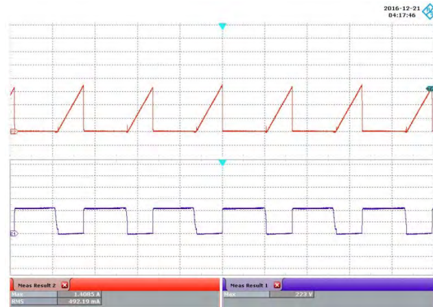
Figure 41 – 100 VAC, 80 V LED Load. Upper: I_{DRAIN} , 400 mA / div. Lower: V_{DRAIN} , 100 V / div., 5 \mu s / div.
