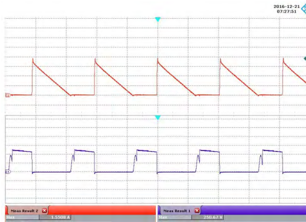
Figure 59 – 115 VAC, 80 V LED Load. Upper: I_{D1} , 400 mA / div. Lower: V_{D1} , 100 V / div., 4 \mu s / div.
