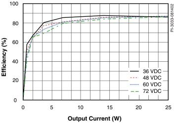
Figure 2. Efficiency vs. Output Power.
