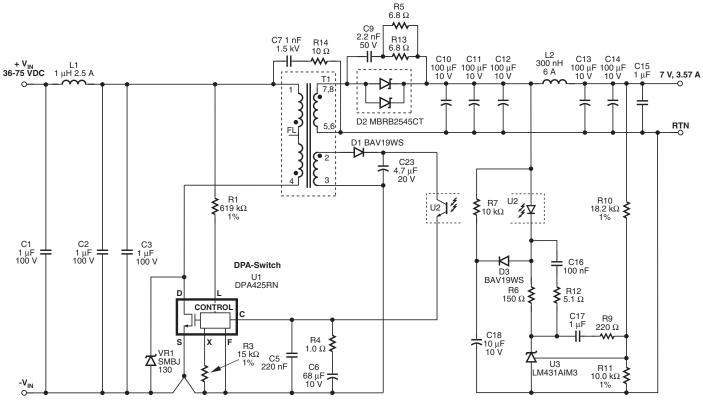
Figure 1. DPA-Switch Flyback DC-DC Converter Schematic.
