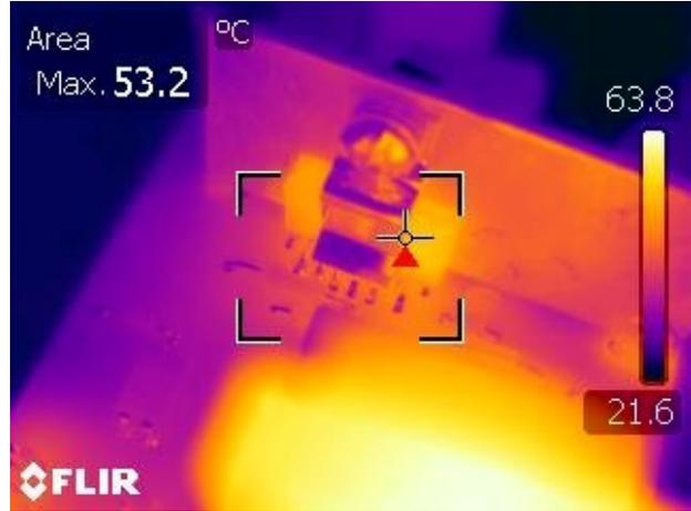
**Figure 58** – Full Load HiperLCS Thermal View, Room Temperature.
