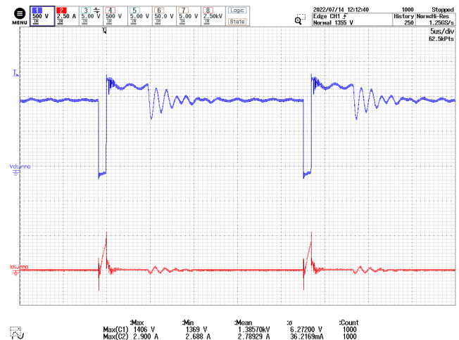
Figure 58 – InnoSwitch3-AQ Drain Voltage and Current. 400 V DC , 2.333 A Load, 25 °C Ambient. CH1: V DS(1C1) , 500 V / div. CH2: I D(1C1) , 2.5 A / div. Time: 5 μs / div.
