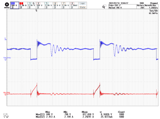
Figure 58 – InnoSwitch3-AQ Drain Voltage and Current. 400 V DC , 2.333 A Load, 25 °C Ambient. CH1: V DS(1C1) , 500 V / div. CH2: I D(1C1) , 2.5 A / div. Time: 5 μs / div.
