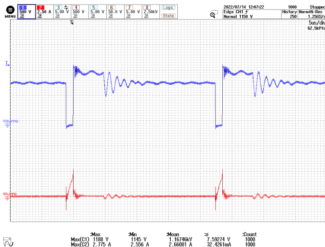
Figure 57 – InnoSwitch3-AQ Drain Voltage and Current. 80 V DC , 2.333 A Load, 25 °C Ambient. CH1: V DS(1C1) , 500 V / div. CH2: I D(1C1) , 2.5 A / div. Time: 5 μs / div.
