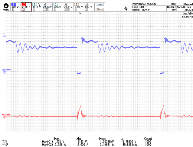
Figure 49 – InnoSwitch3-AQ Drain Voltage and Current. 80 V DC , 2.333 A Load, 85 °C Ambient. CH1: V_{DS(IC1)} , 500 V / div. CH2: I_{D(IC1)} , 2.5 A / div. Time: 5 μs / div.
